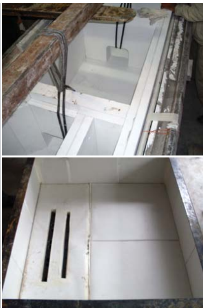
Far left, top and bottom left: samples of Microtherm high performance insulation material employed at Chemco Harapan's furnaces with Promat ALSIFLEX®-1260, MONOLITE® M1 and MICROTHERM® SG.
