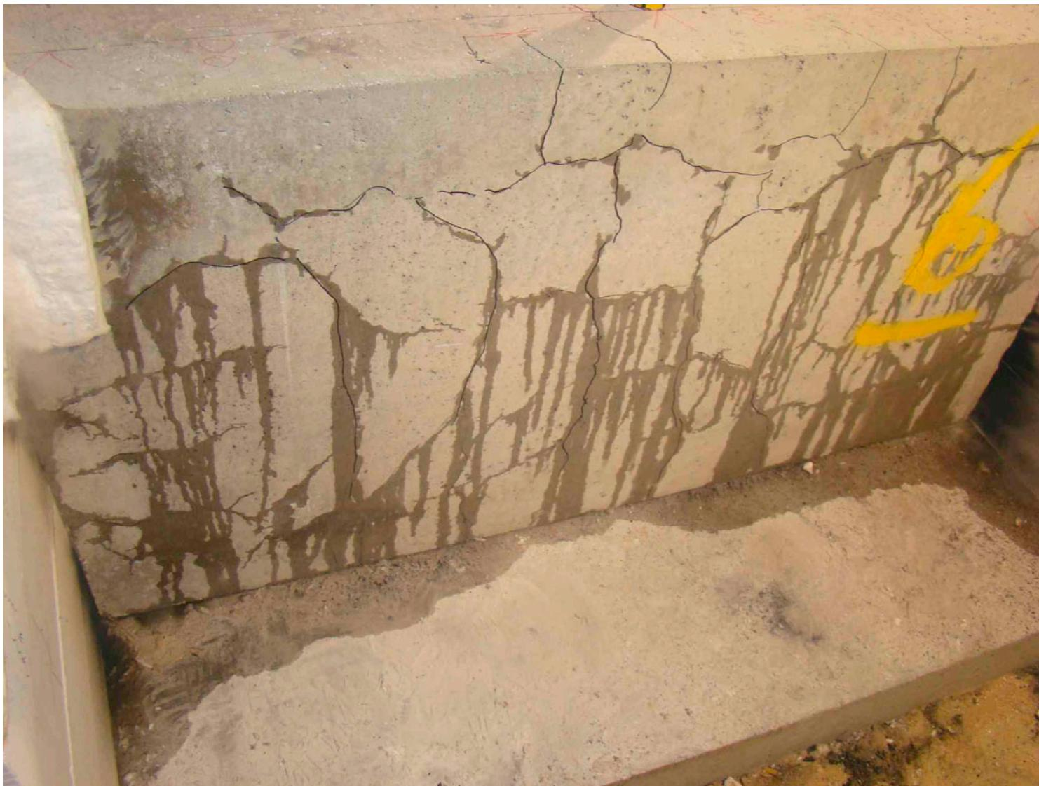
Figure B16 Element 6 after 40 minutes of heating
