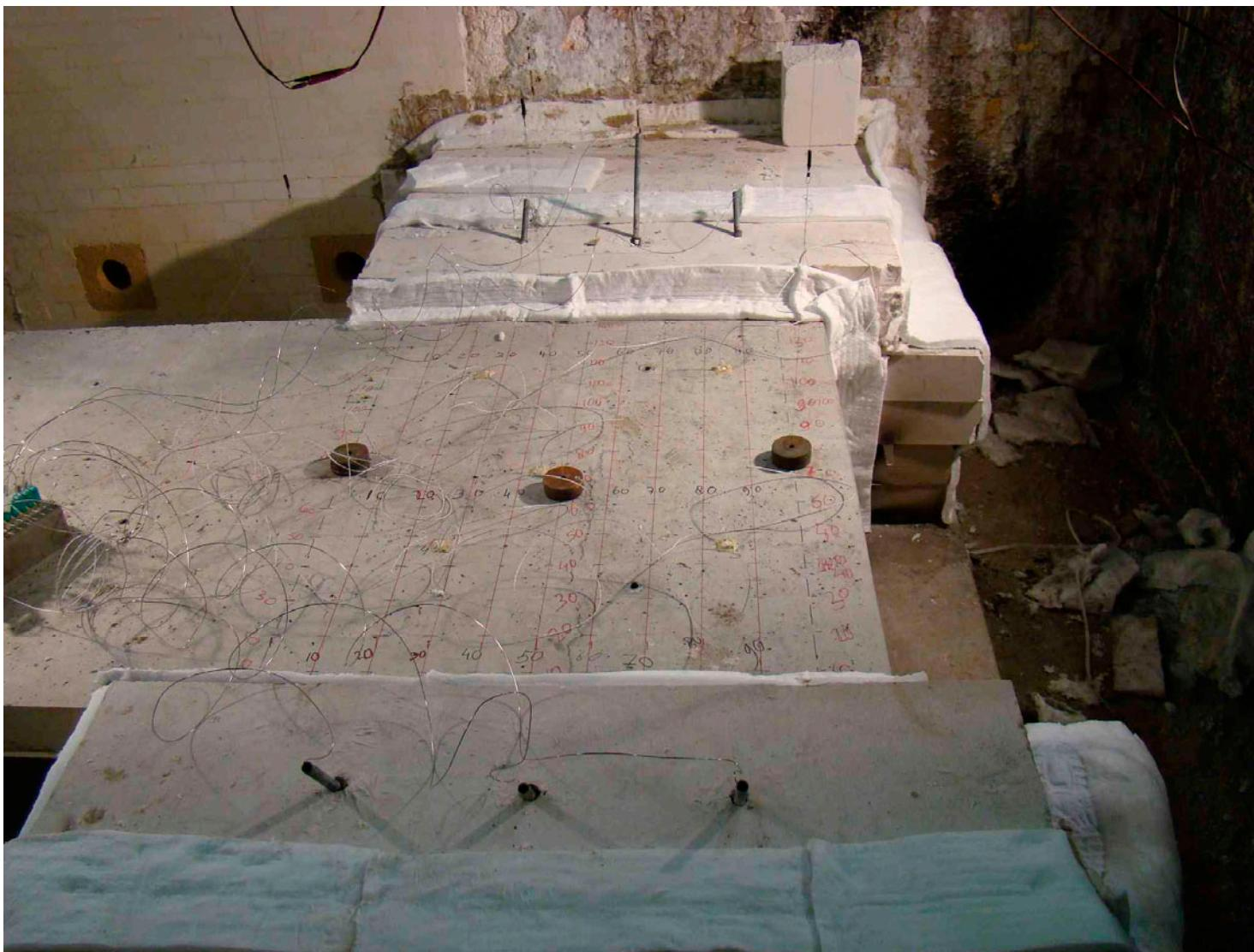
Figure G4 Element 9 before the fire test
