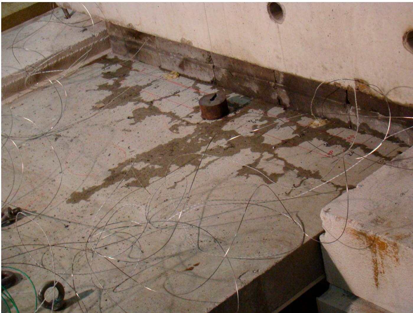
Figure I8 Element 7 after 75 minutes of heating
