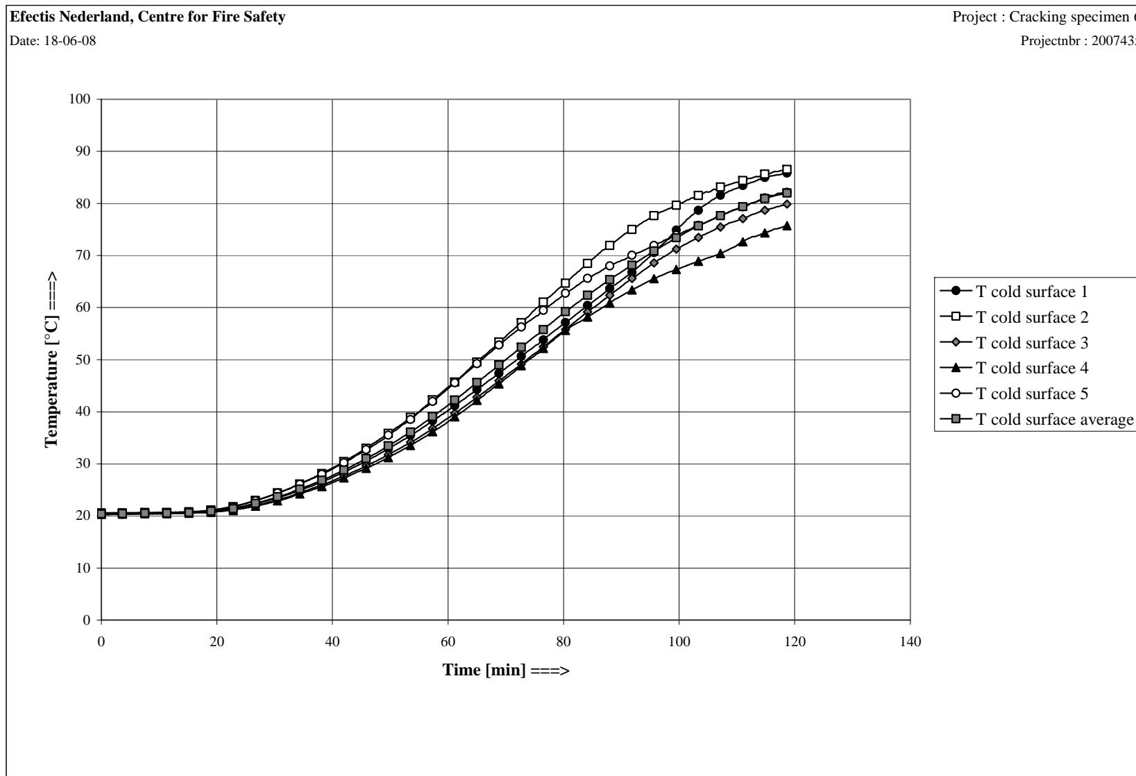
Figure B2 Cold surface temperatures
