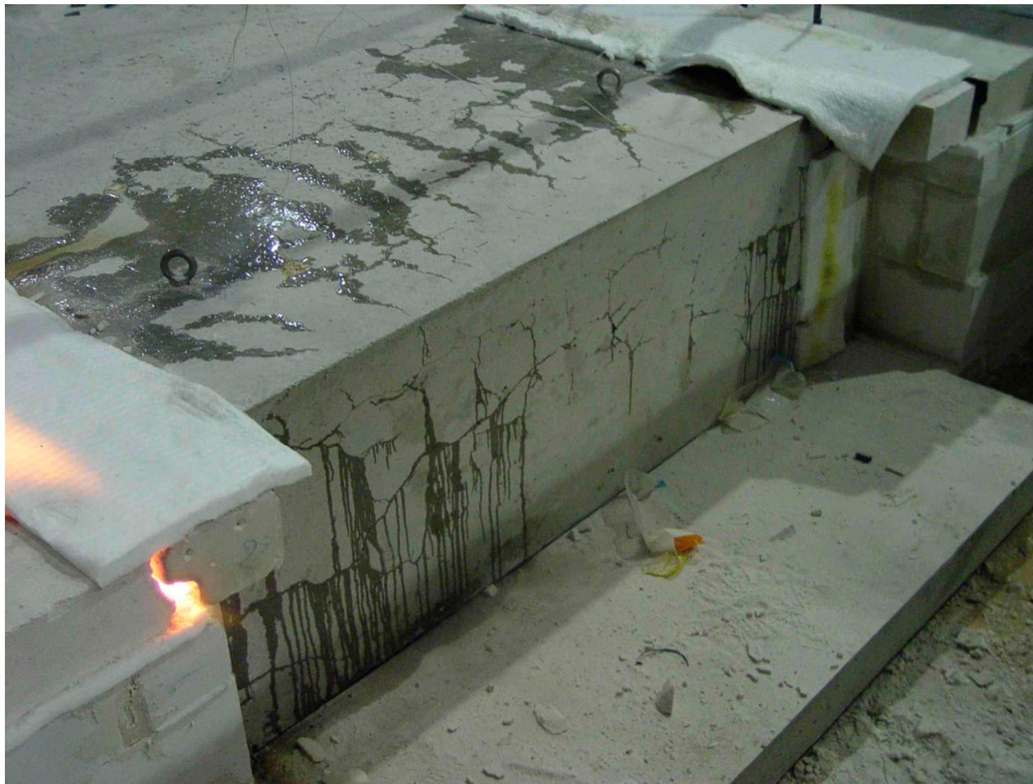
Figure A4 Element 0 after 13 minutes of heating
