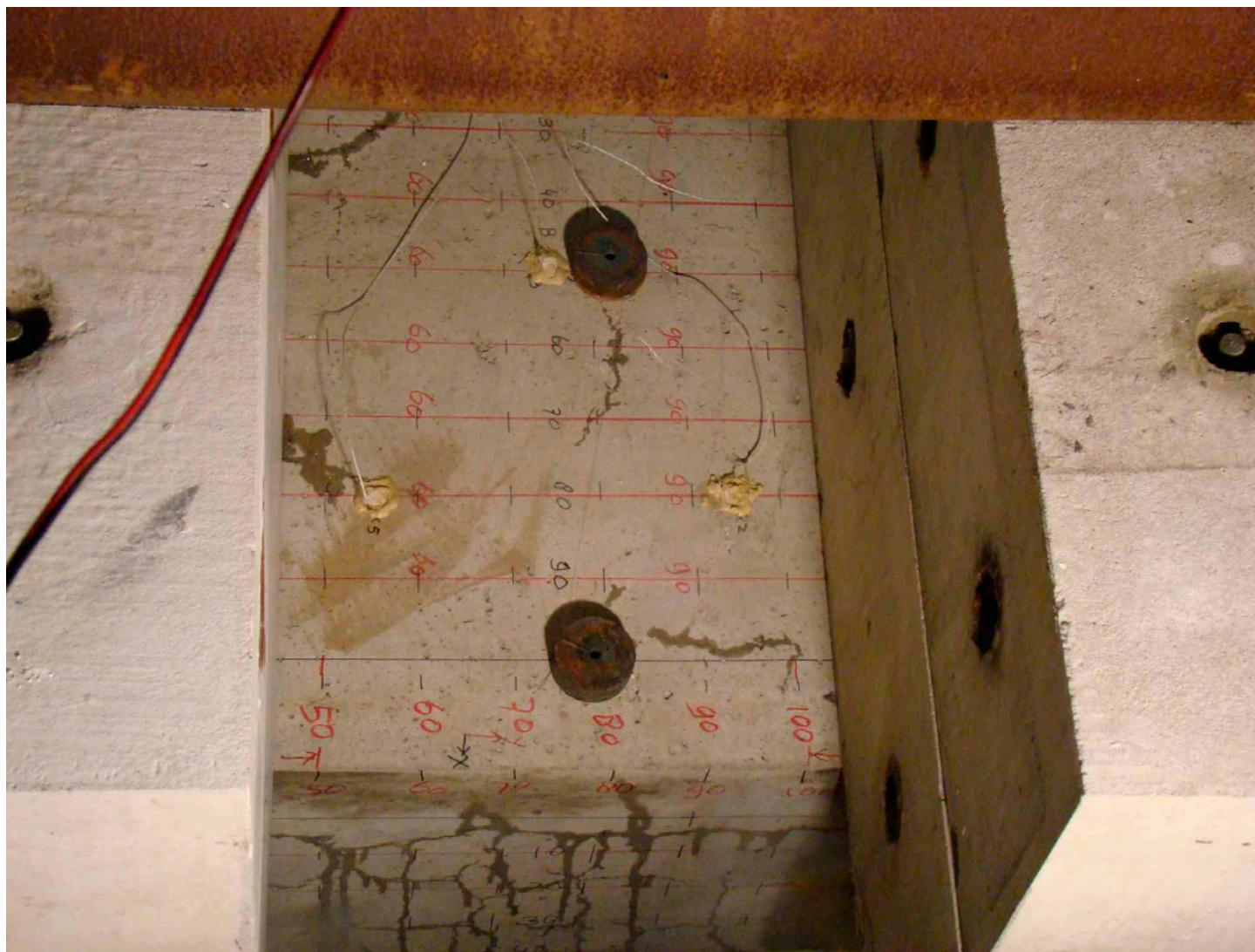
Figure E10 Element 6 after 61 minutes of heating
