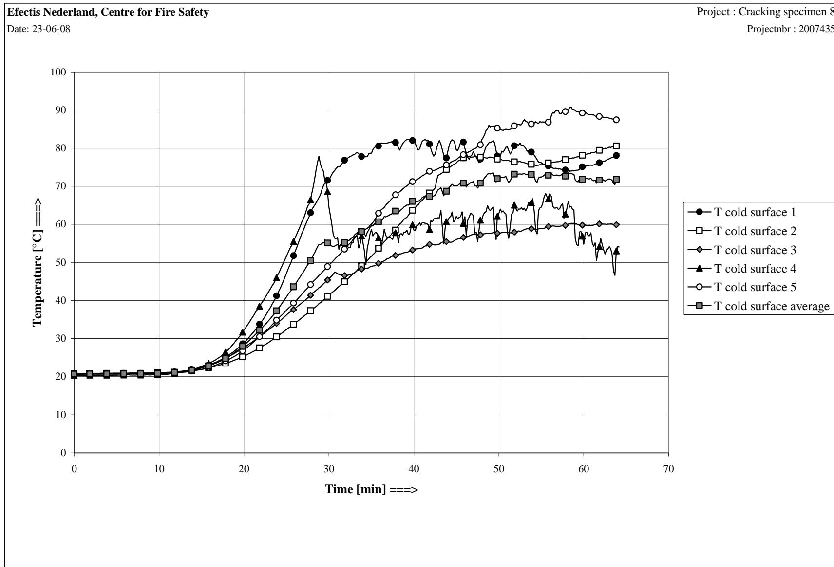
Figure D2 Cold face temperatures
