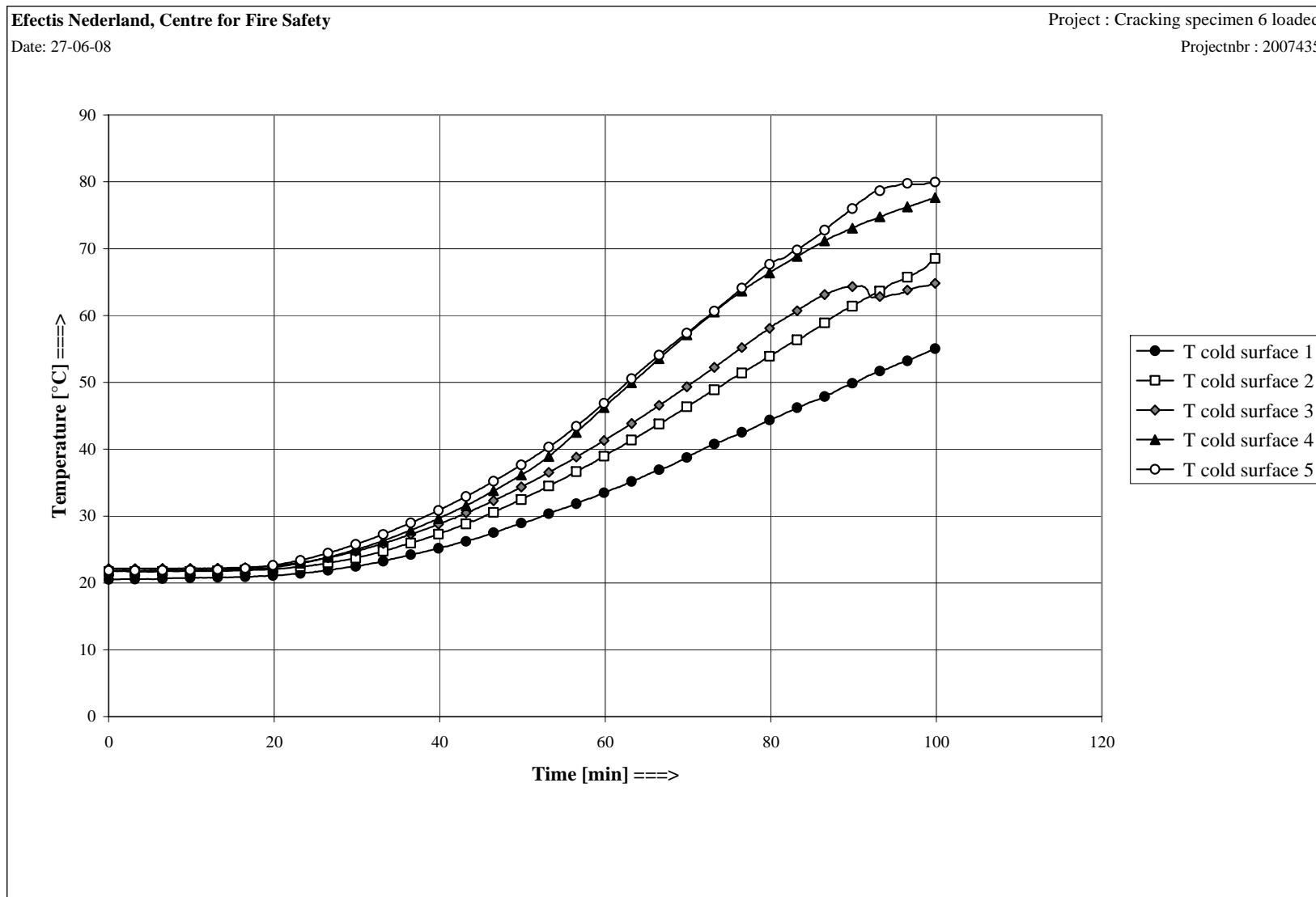
Figure E2 Cold face temperatures
