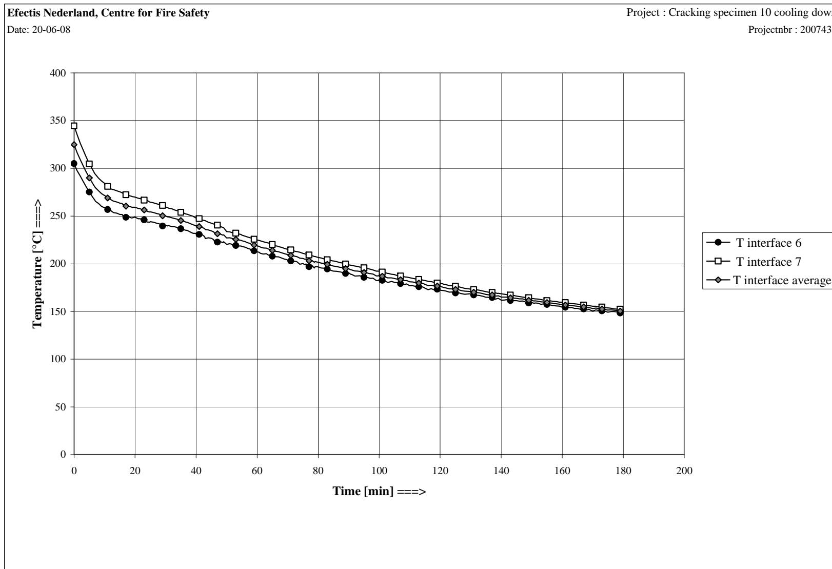
Figure C7 Interface temperatures during cooling down
