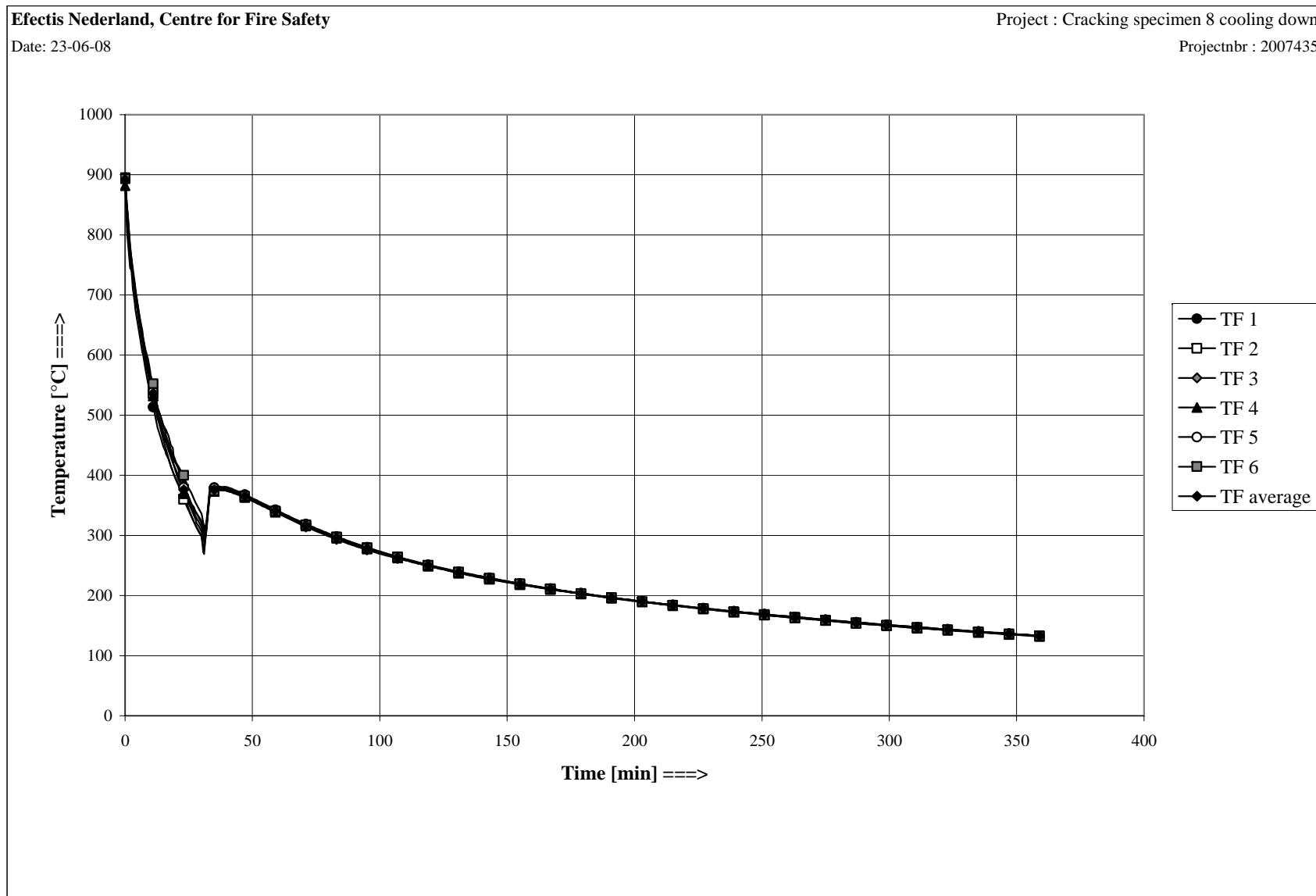
Figure D4 Furnace temperature during cooling down
