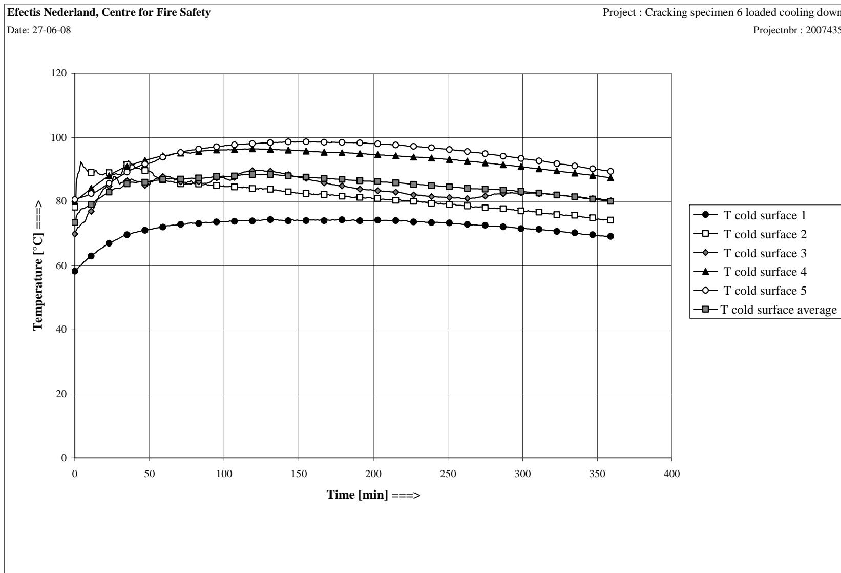
Figure E6 Cold surface temperatures during cooling down
