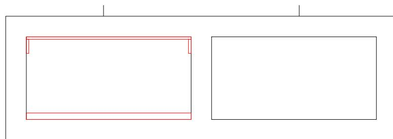
Figure 4.1 Locations of the Promatect-H® lining on the ceiling and walls and its fixation locations
