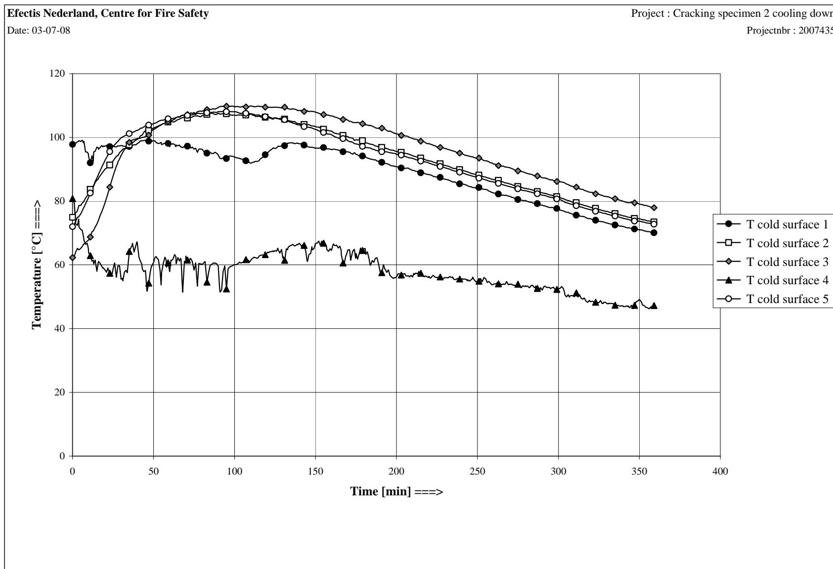
Figure F5 Cold face temperatures during cooling down
