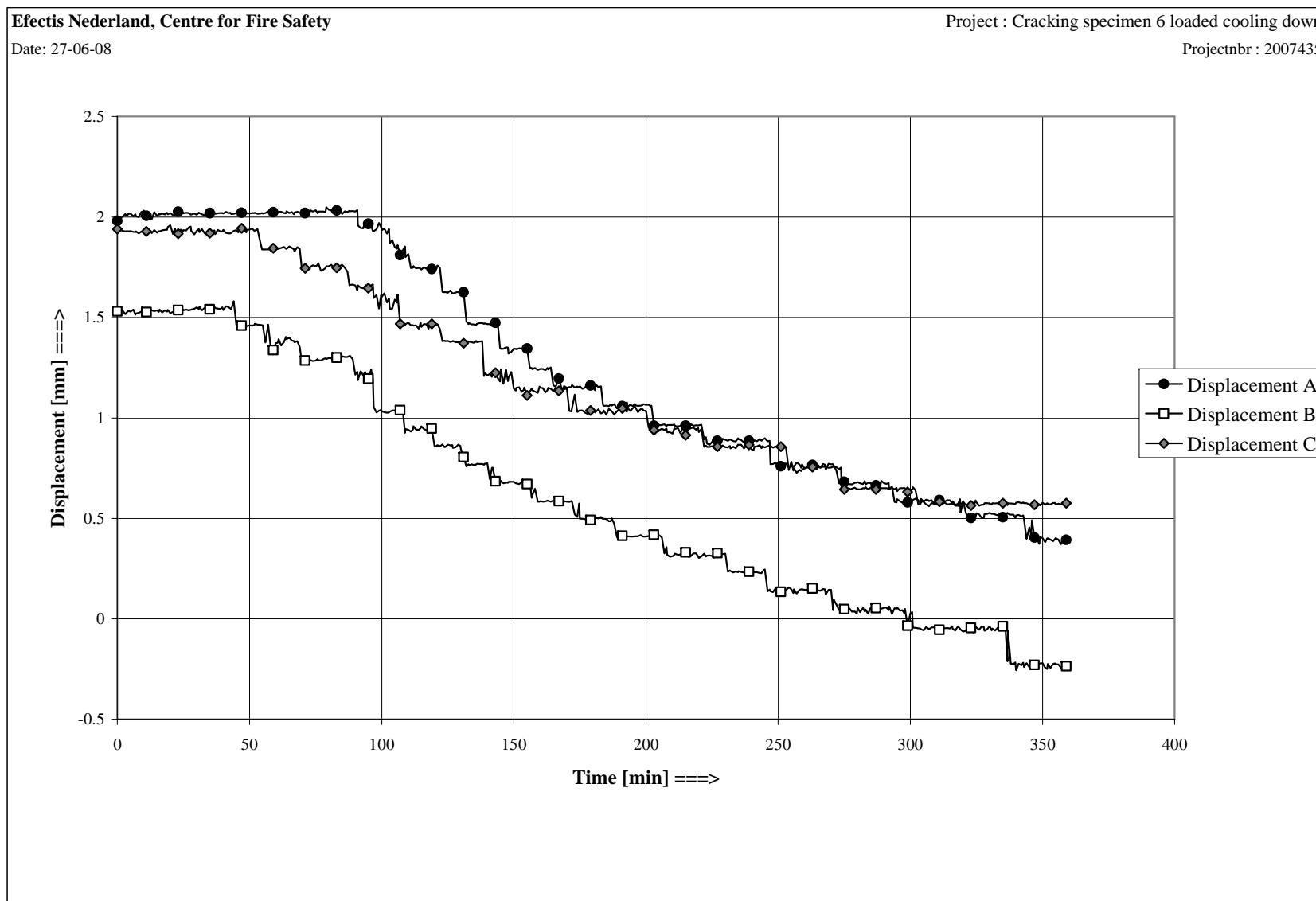
Figure E8 Displacements of the cold surface during cooling down
