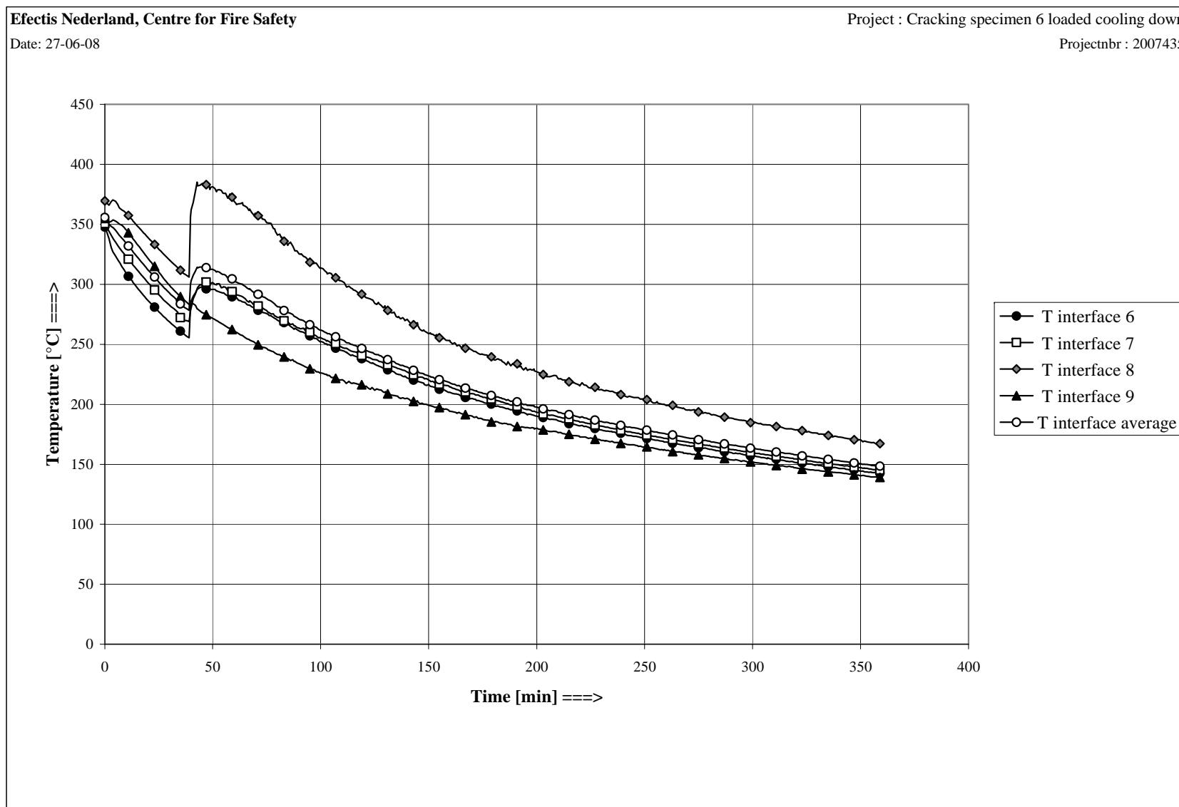
Figure E7 Interface temperatures during cooling down
