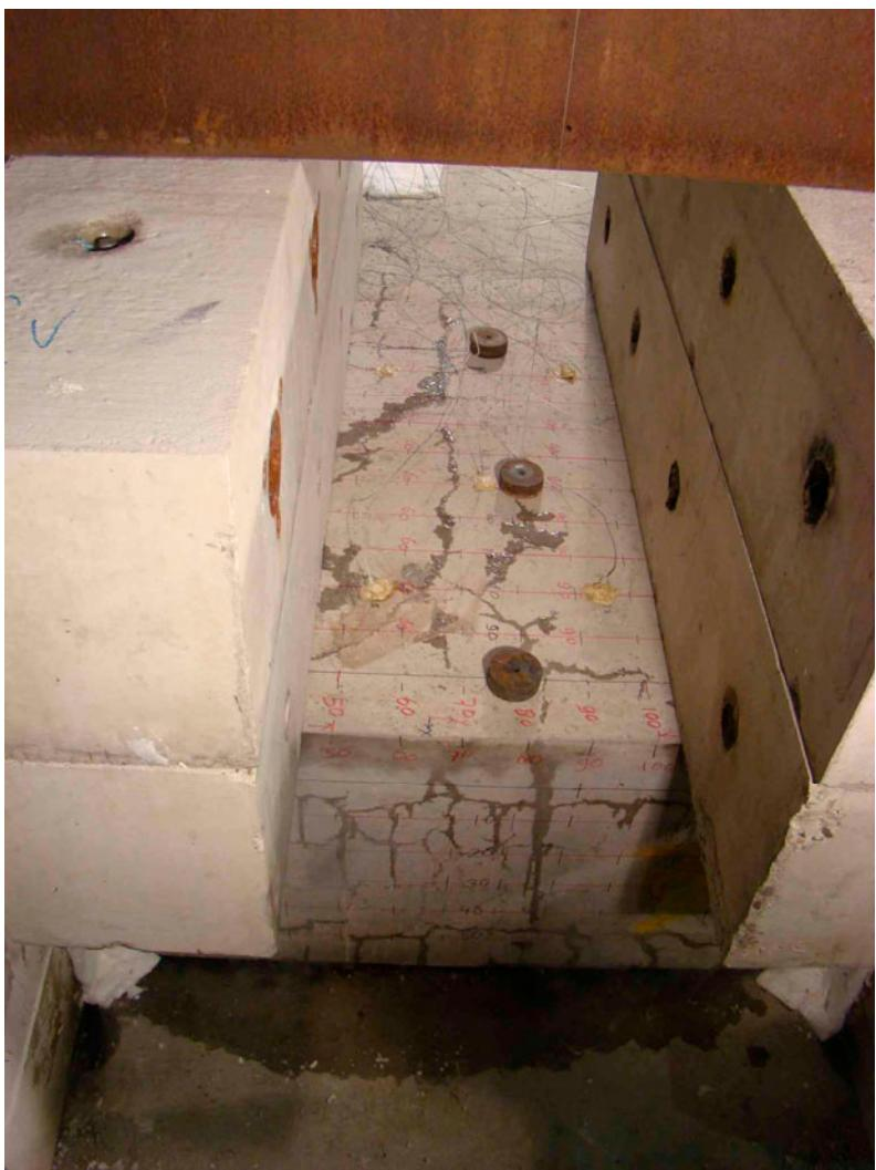
Figure E11 Element 6 after 78 minutes of heating
