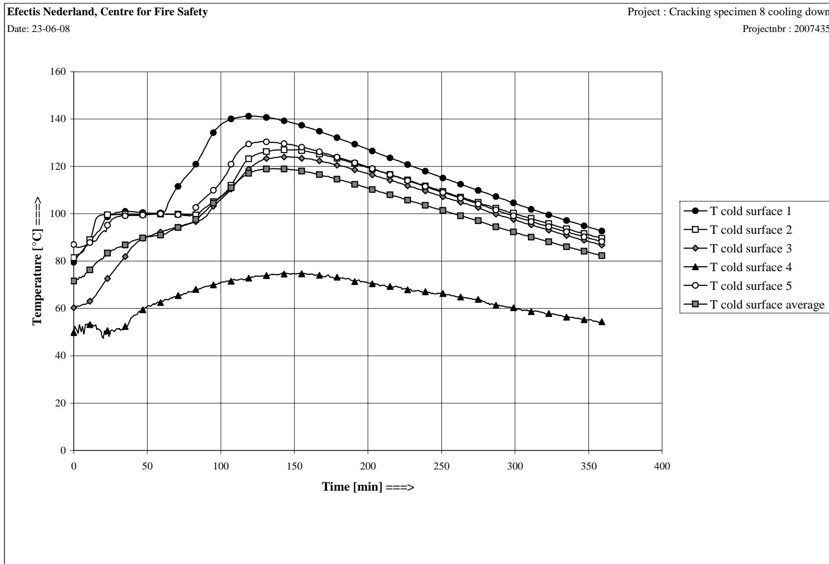
Figure D5 Cold surface temperatures during cooling down
