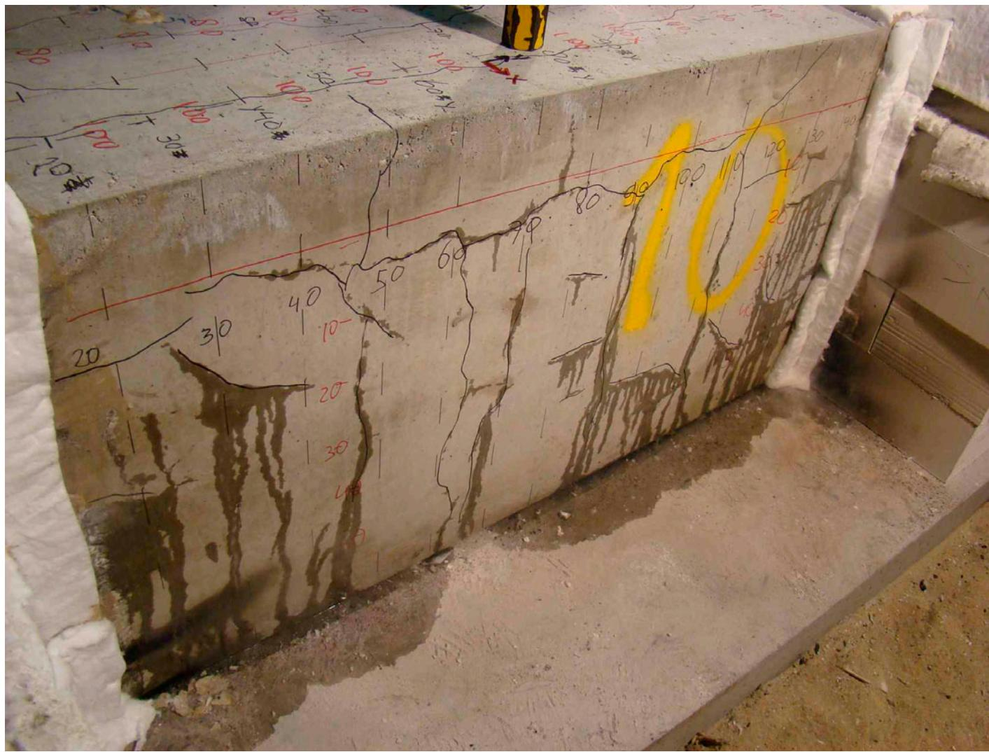
Figure C12 Element 10 after 29 minutes of heating, view on the side surface
