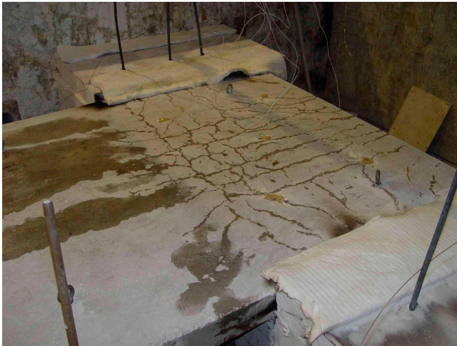
Figure A8 Element 0 after 56 minutes of heating
