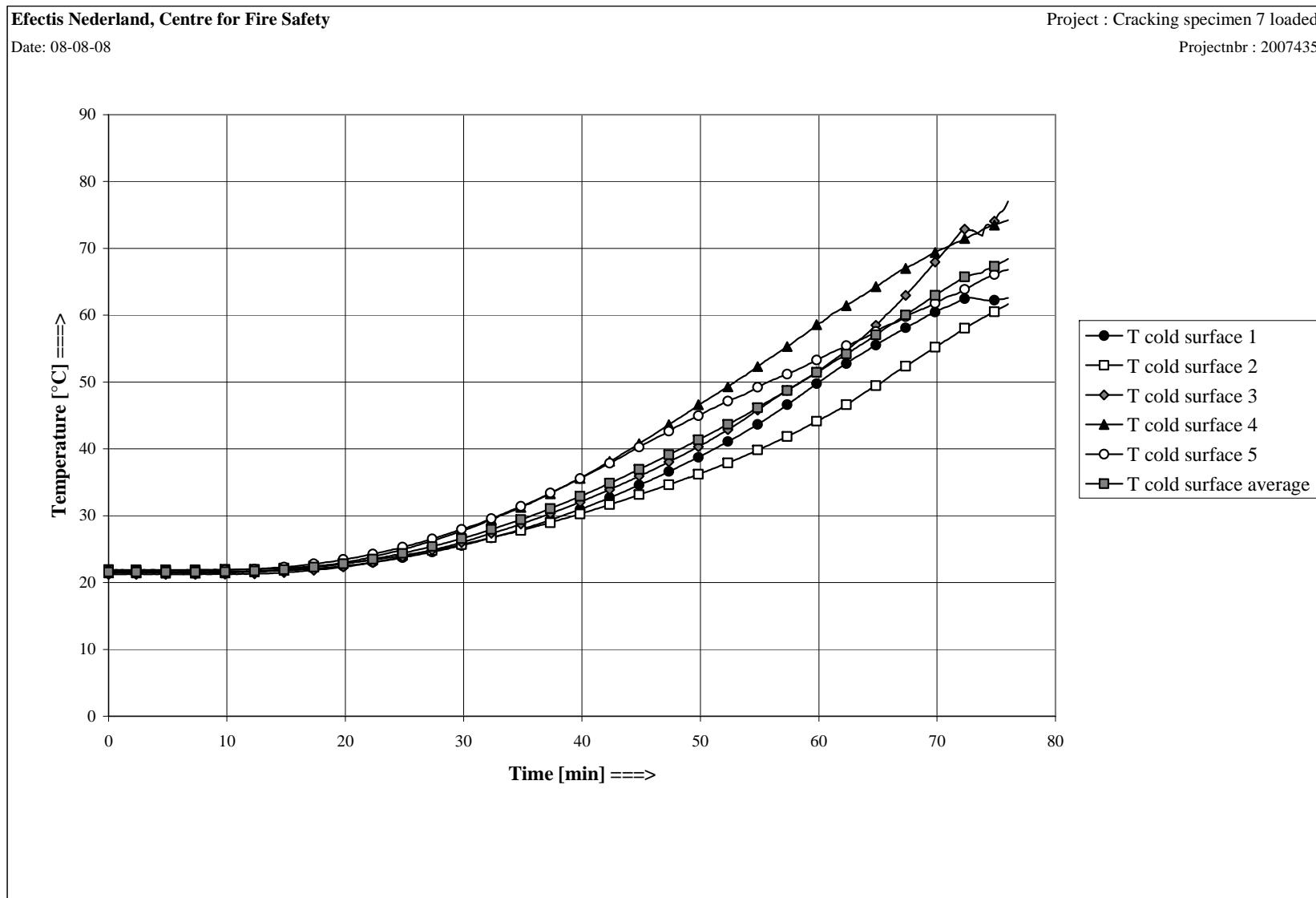
Figure I2 Cold surface temperatures
