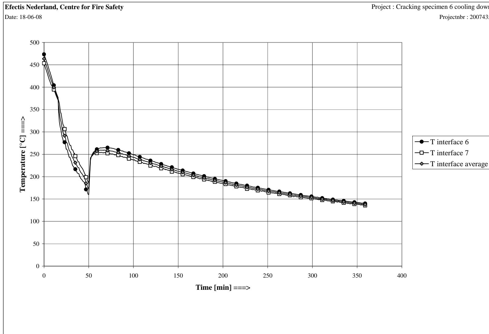
Figure B6 Interface temperatures during cooling down
