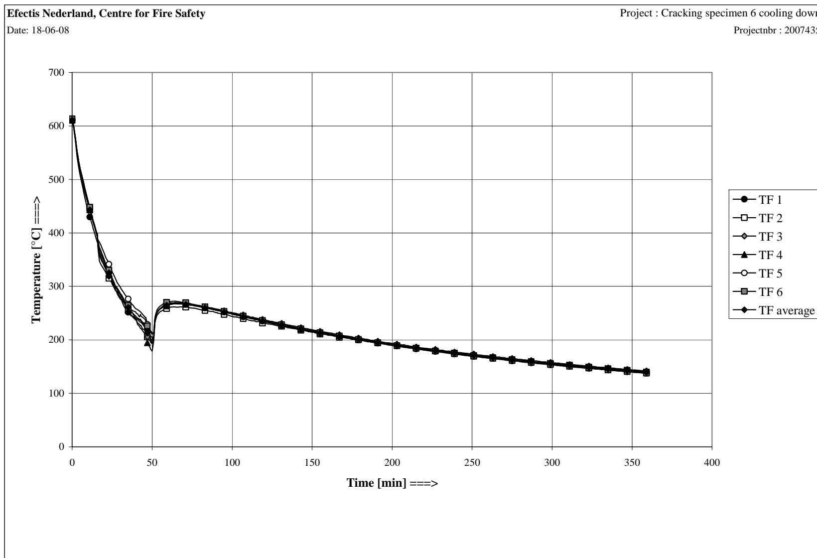
Figure B4 Furnace temperature during cooling down
