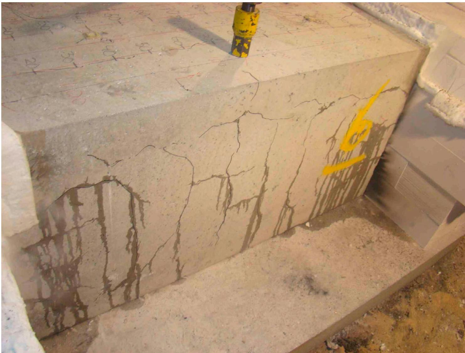
Figure B15 Element 6 after 27 minutes of heating
