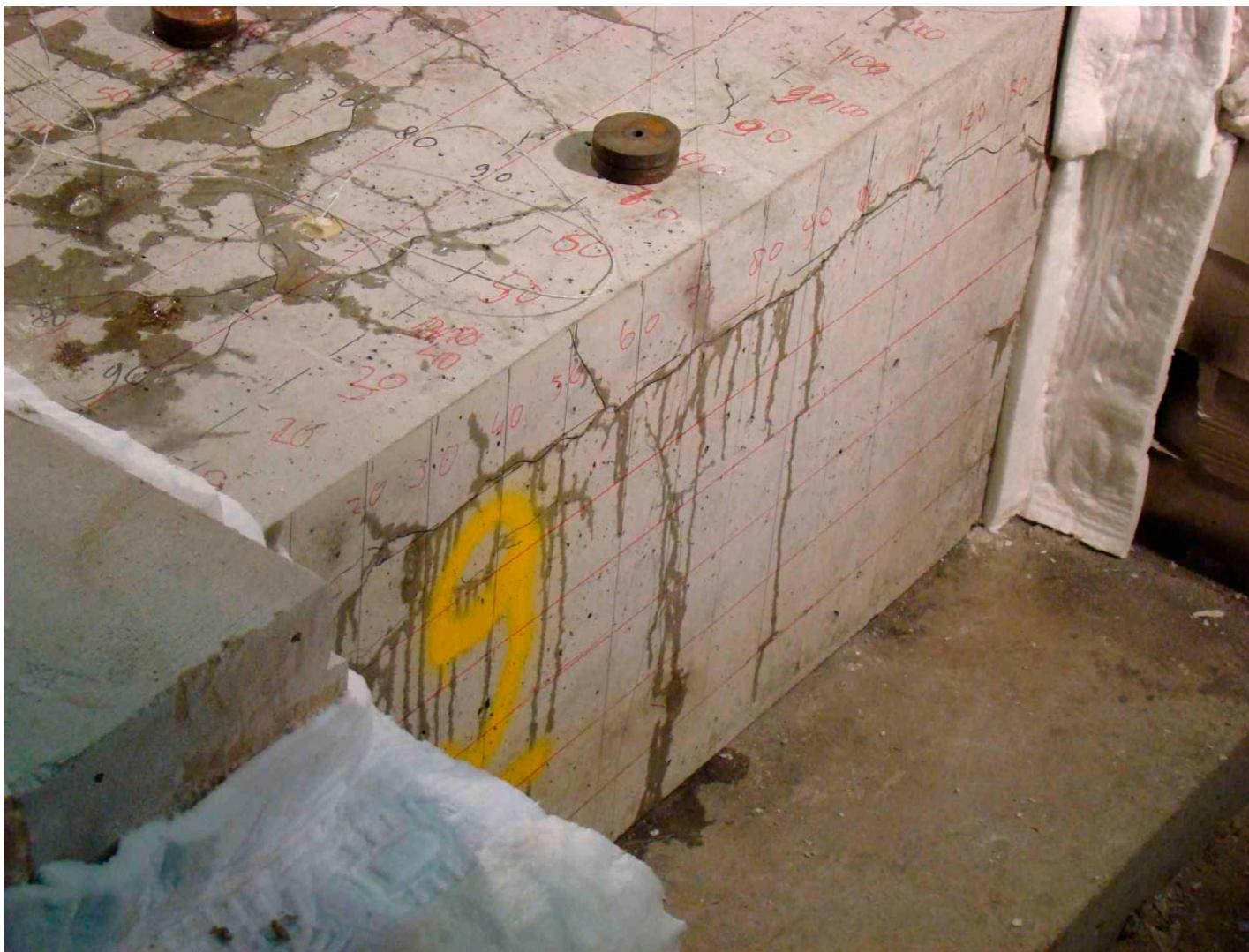
Figure G11 Element 9 after 48 minutes of heating
