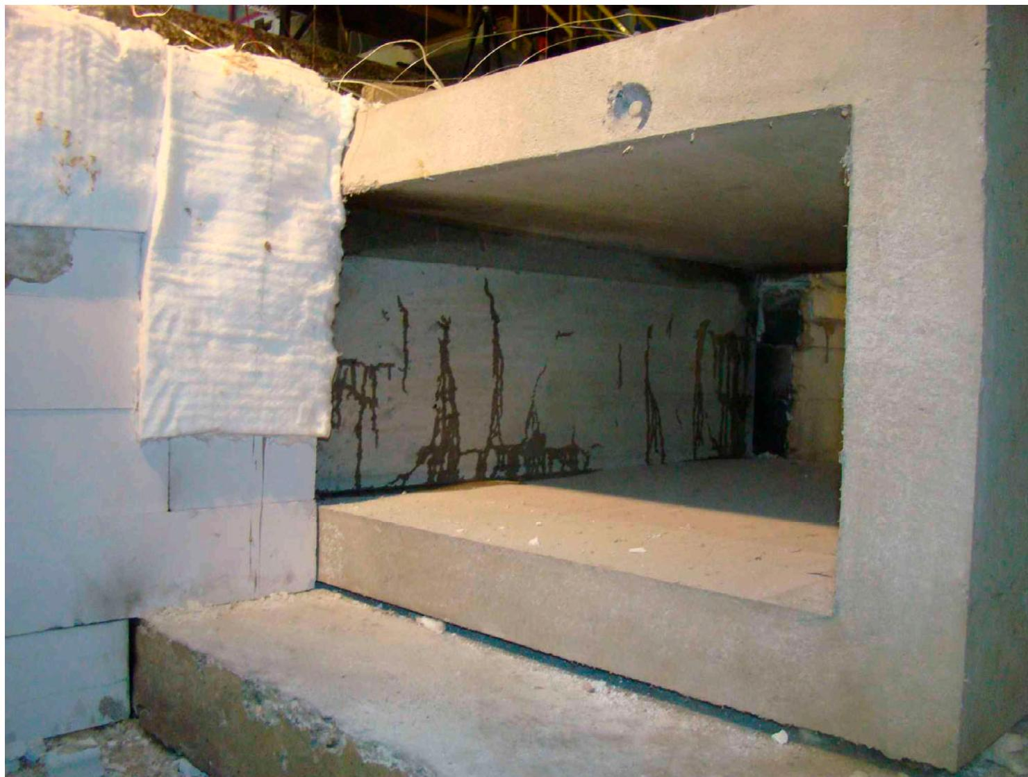
Figure C11 Element 10 after 20 minutes of heating, a view on the non heated tube. Note that the bottom of the element is lifted from the floor
