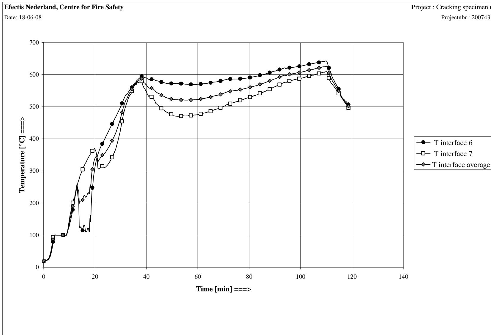
Figure B3 Interface temperatures
