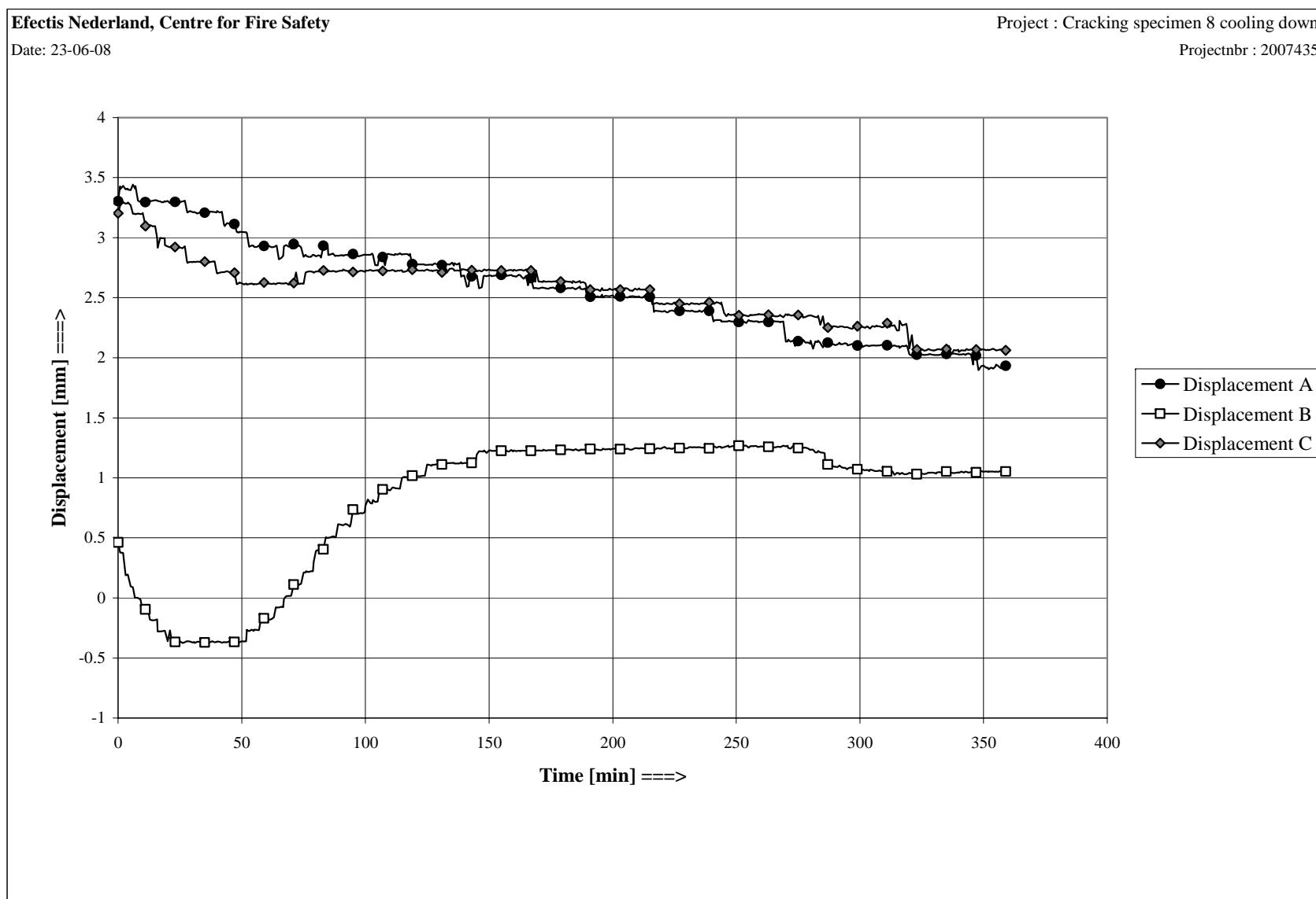
Figure D6 Displacements during cooling down
