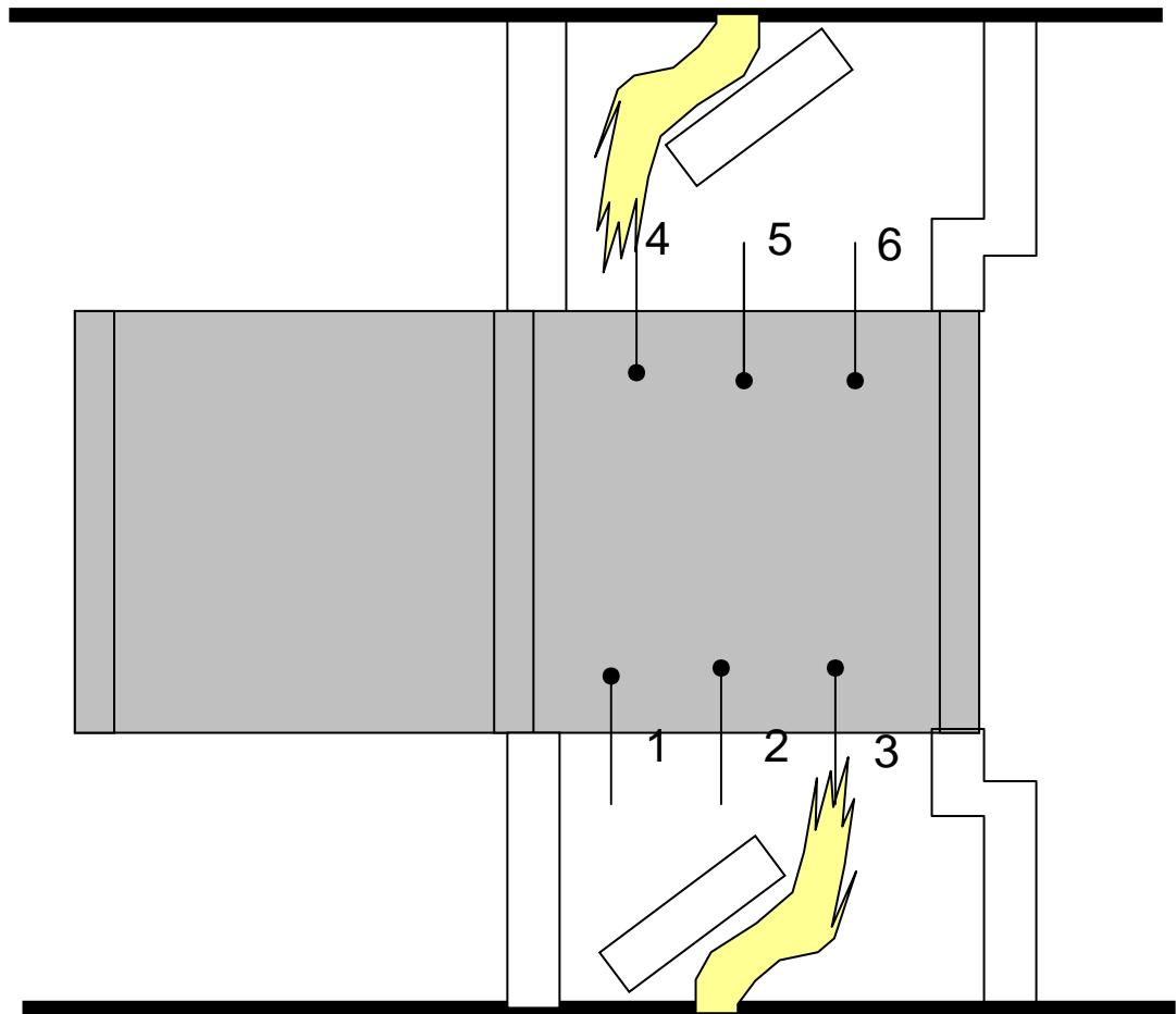
Figure 5.1 Schematic top view of the test set up in the horizontal furnace. The scaled tunnel element is placed in the centre. Around it, an aerated autoclaved concrete compartment was built to create a compartment of the heated tube, the furnace walls, the gas burners and furnace exhaust holes.
