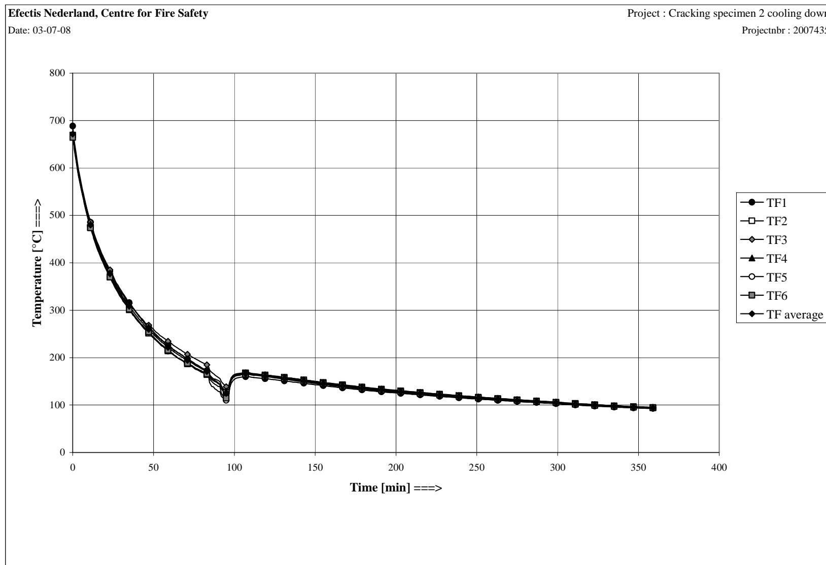
Figure F4 Furnace temperature during cooling down
