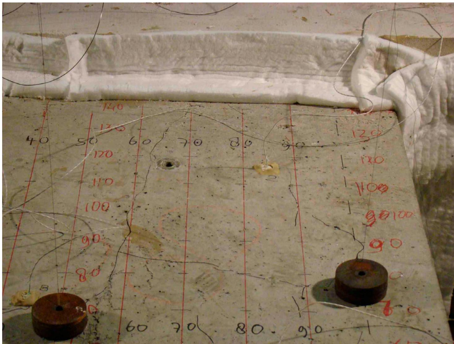
Figure G6 Element 9 after 14 minutes of heating, upper right corner
