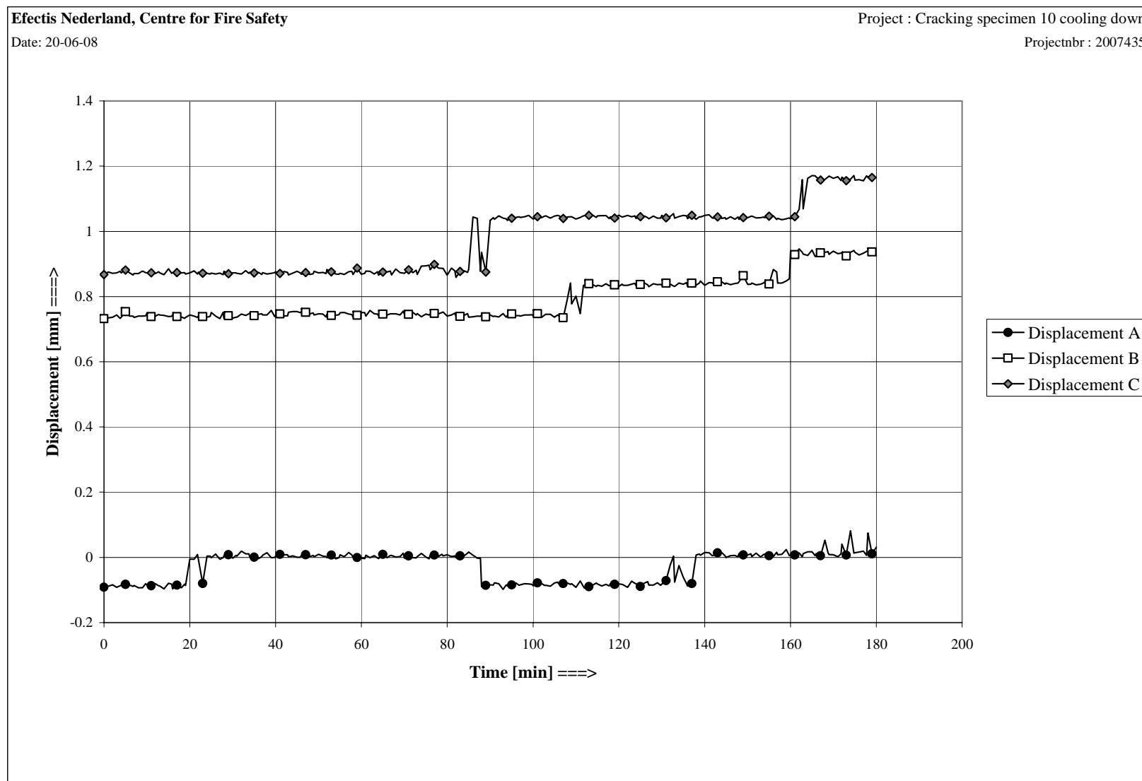
Figure C8 Displacements cold surface during cooling down
