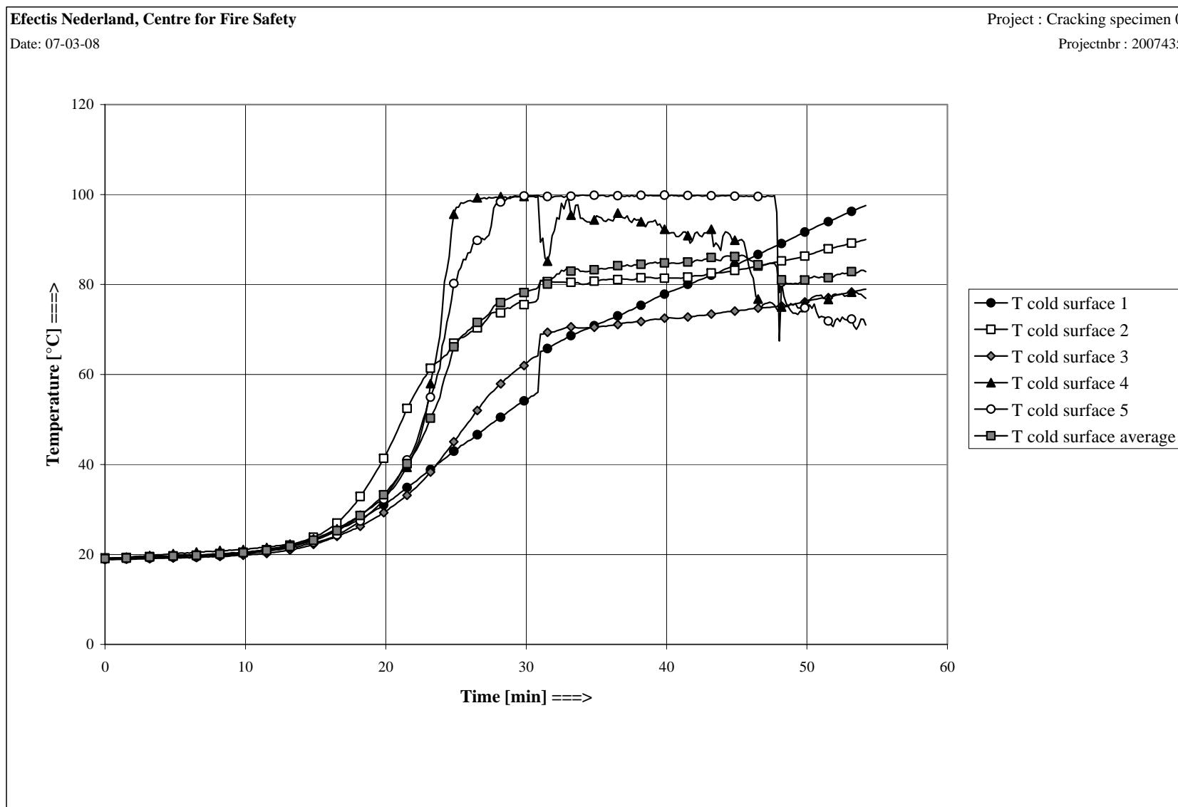
Figure A2 Cold surface temperatures
