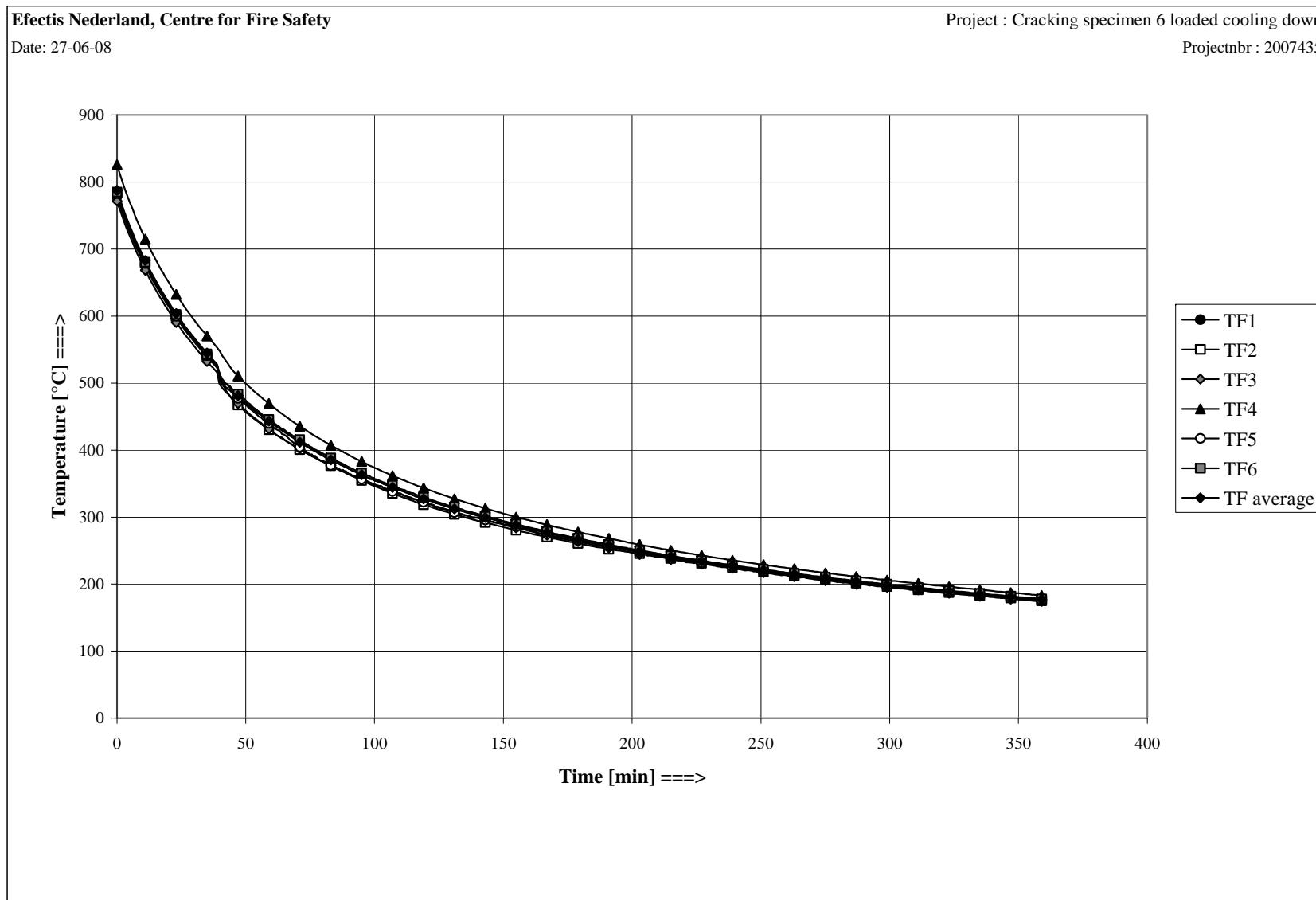
Figure E5 Furnace temperature during cooling down
