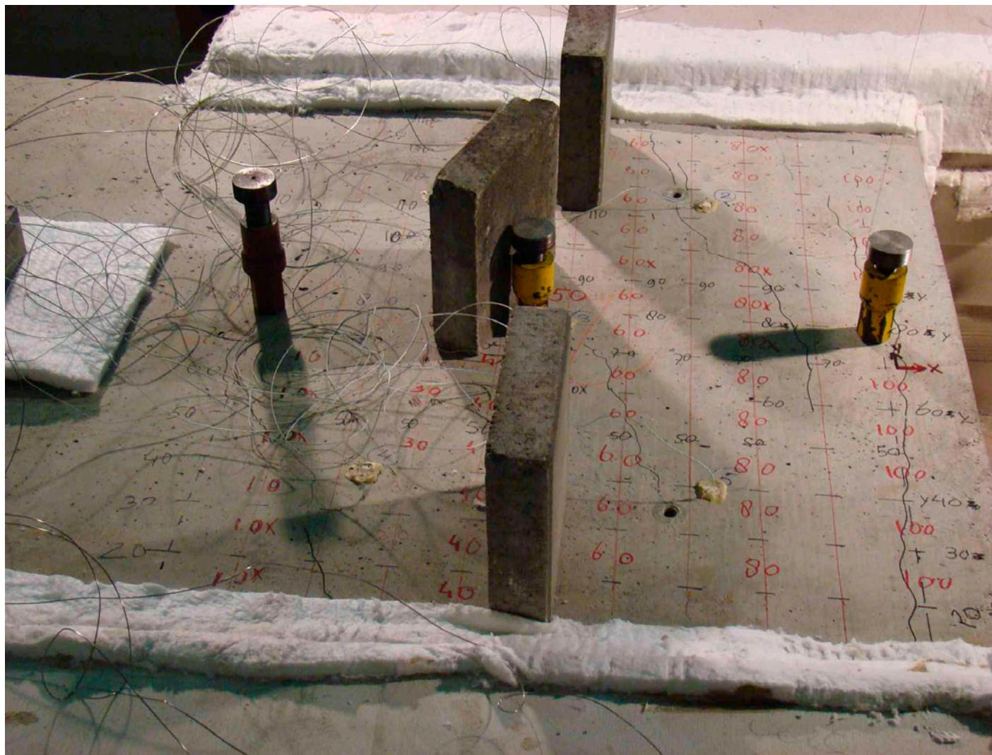
Figure C10 Element 10 after 19 minutes of heating
