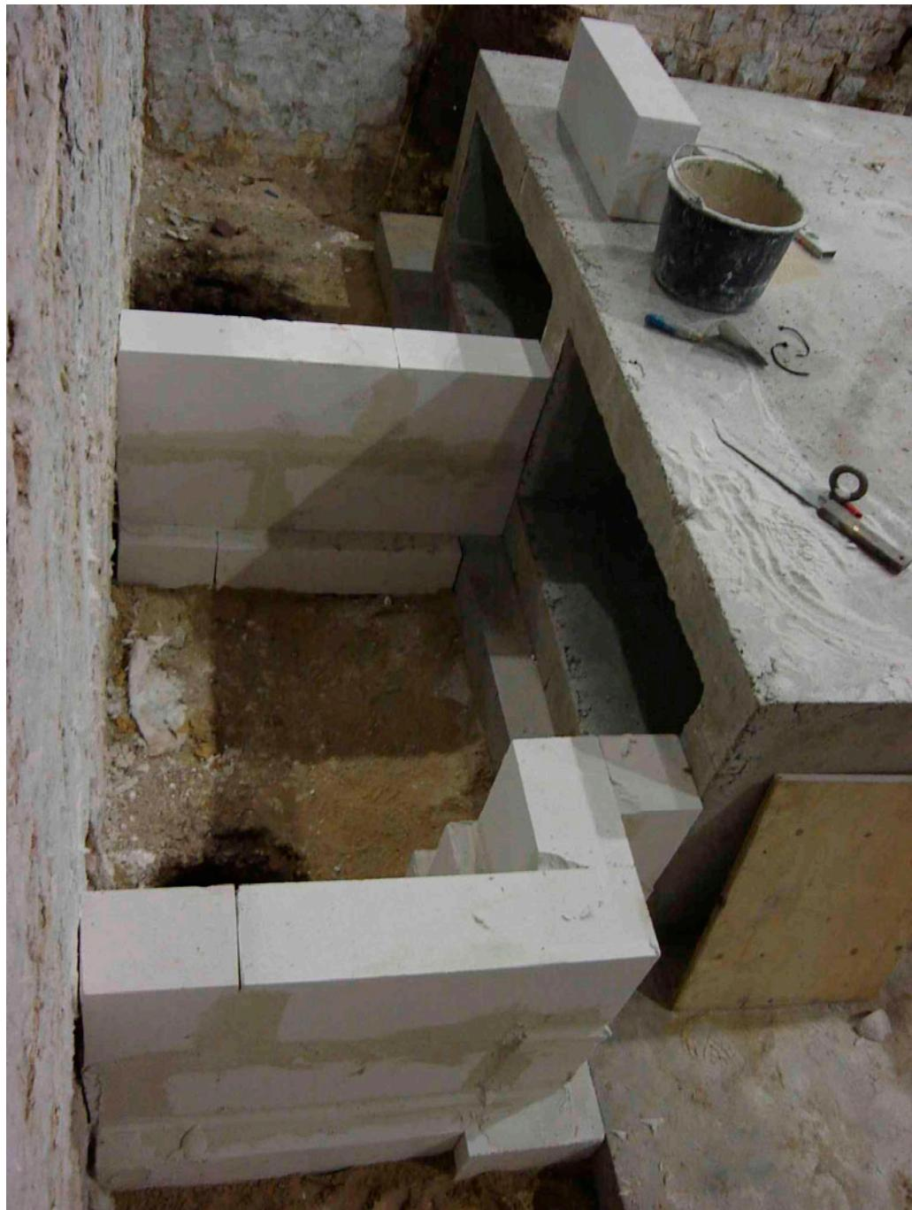
Figure 5.2 Top view of the test set up in the horizontal furnace.
