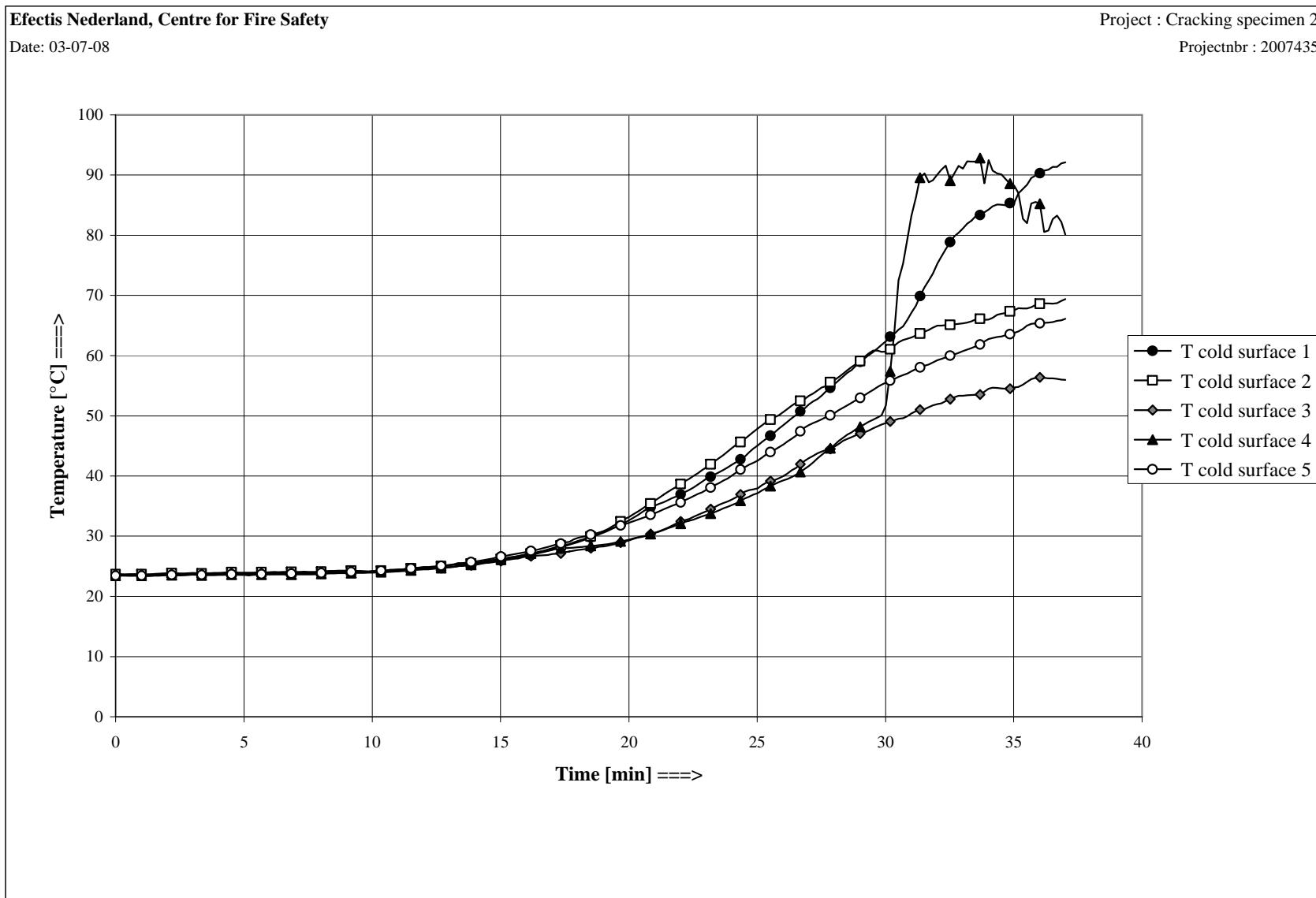
Figure F2 Cold face temperatures
