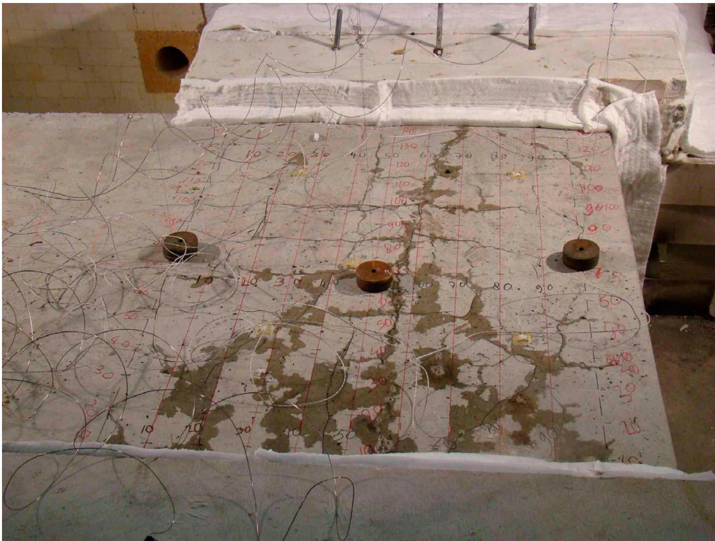
Figure G10 Element 9 after 45 minutes of heating
