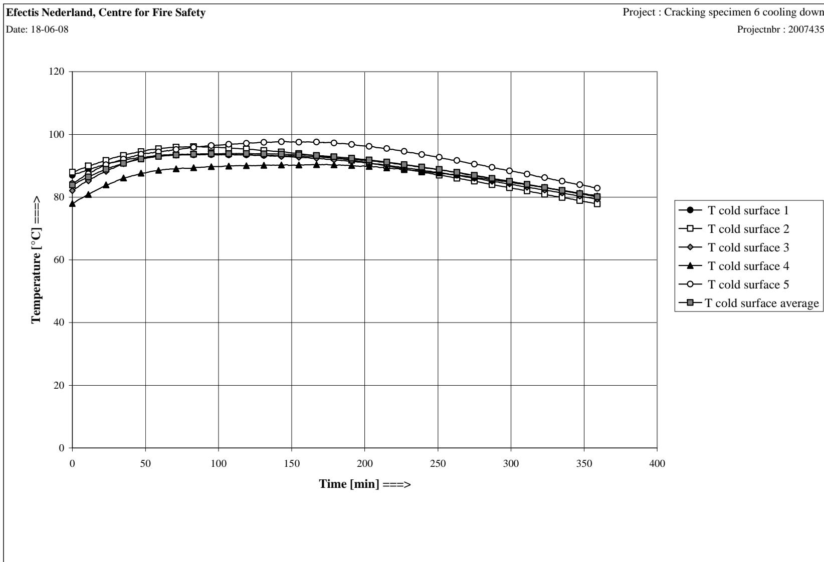
Figure B5 Cold surface temperatures during cooling down
