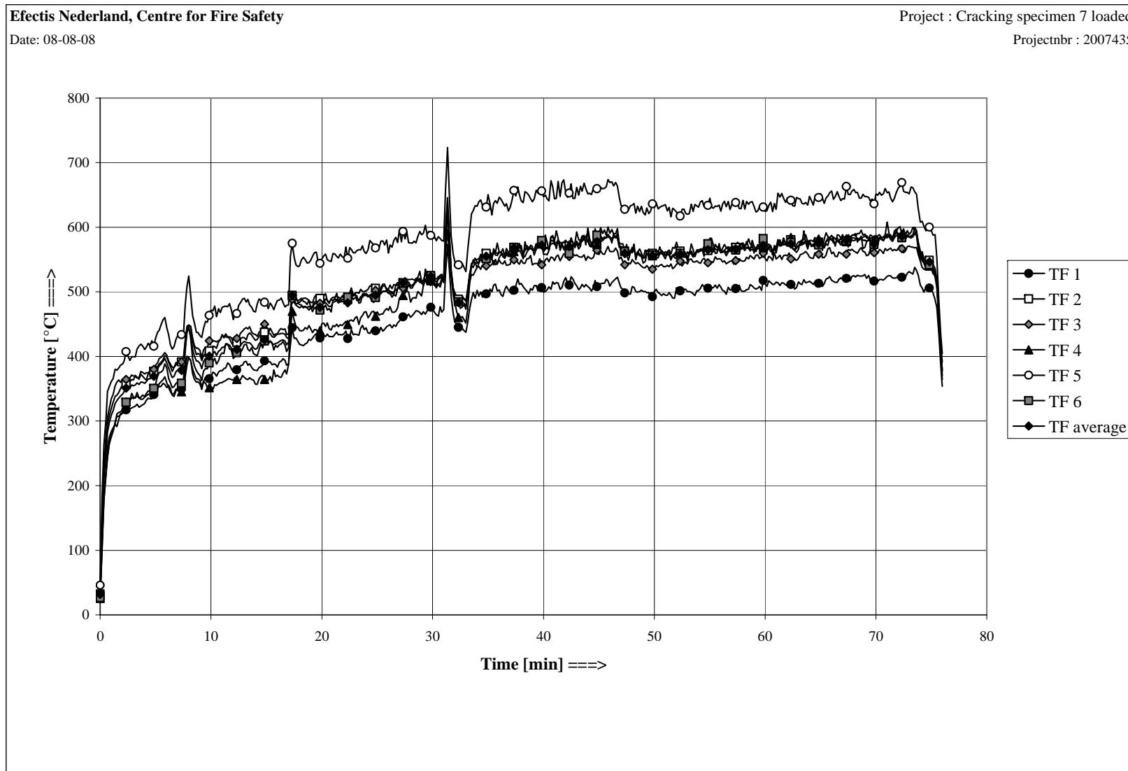
Figure I1 Furnace temperatures
