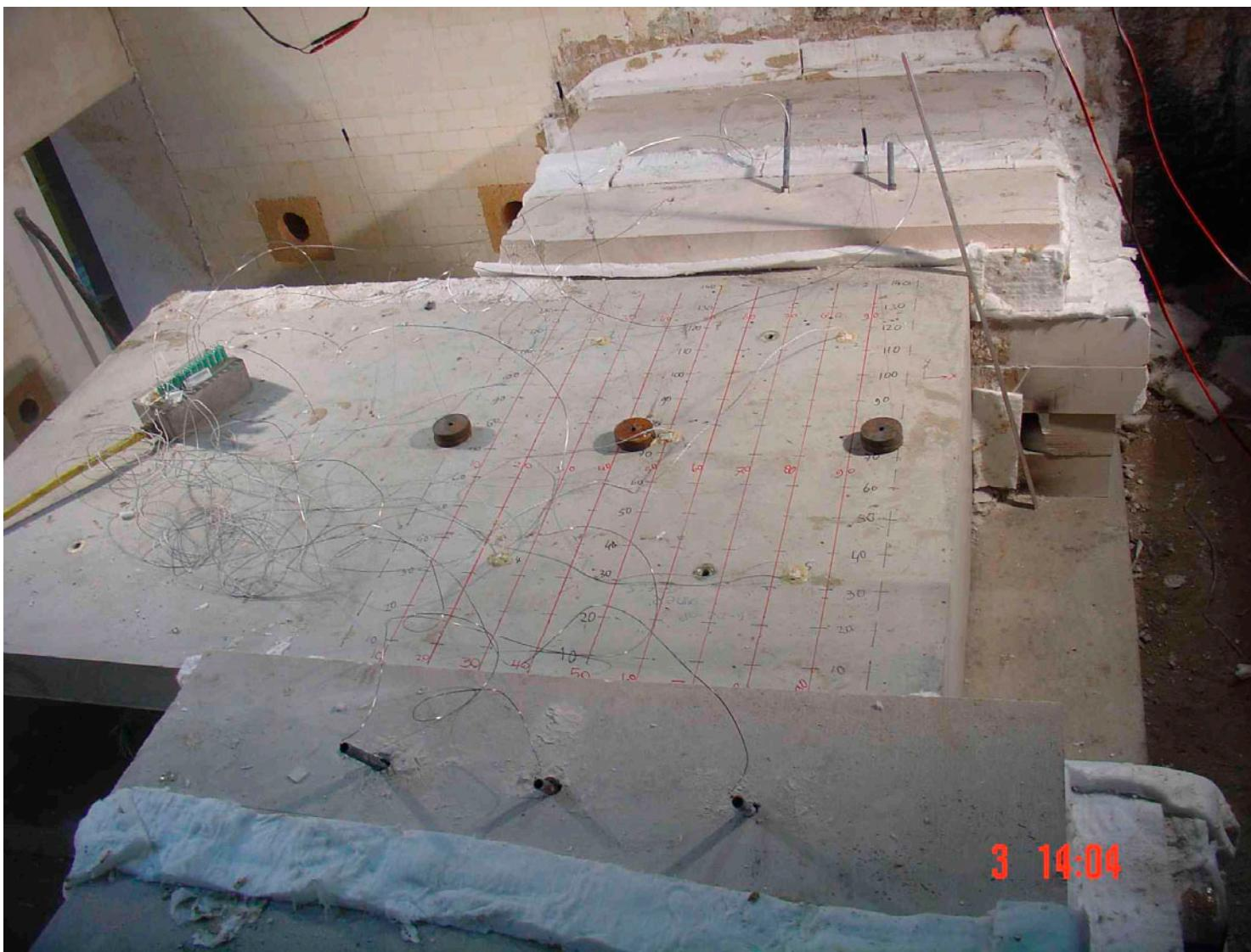
Figure F7 Element 2 before the fire test
