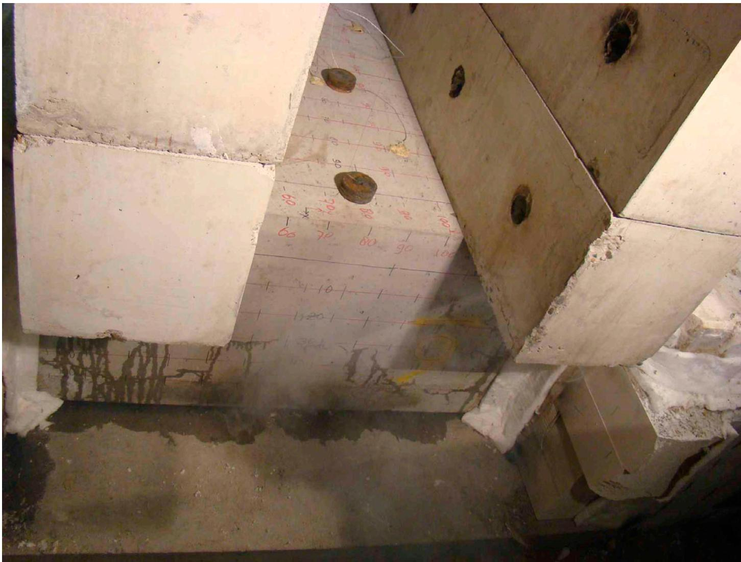
Figure E10 Element 6 after 28 minutes of heating
