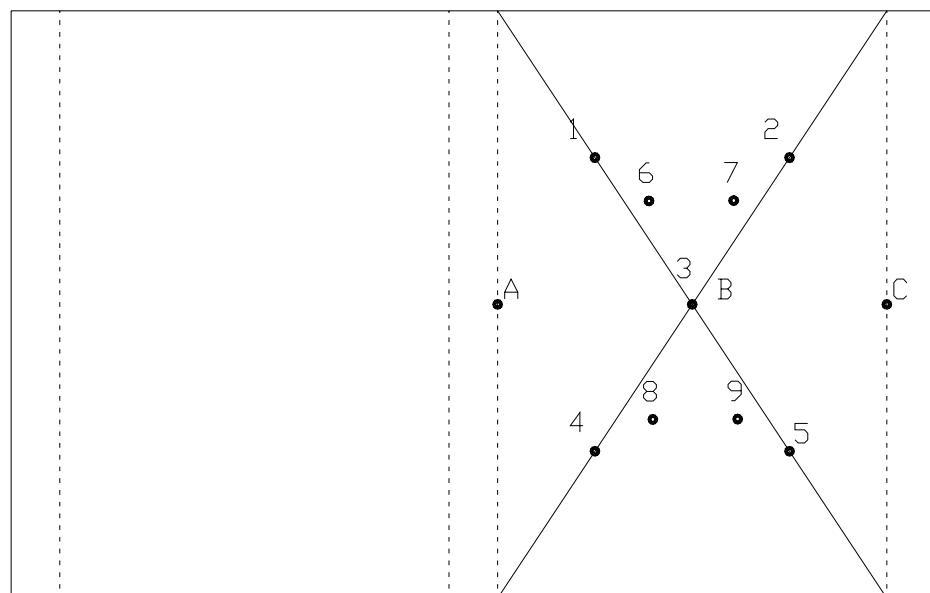
Figure 5.5 Overview of the thermocouples on the cold surface, 1 to 5, the interface temperature 6 to 9 and the displacement measurement locations A, B and C
