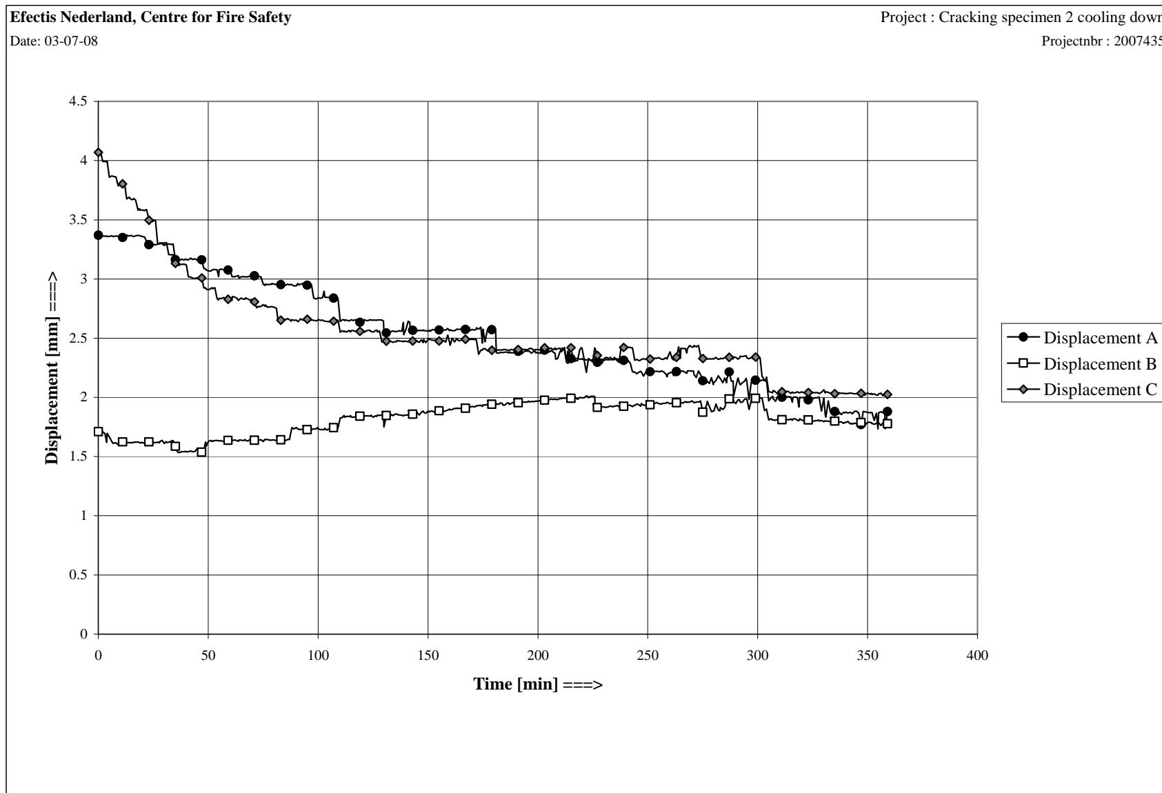
Figure F6 Displacements cold surface during cooling down
