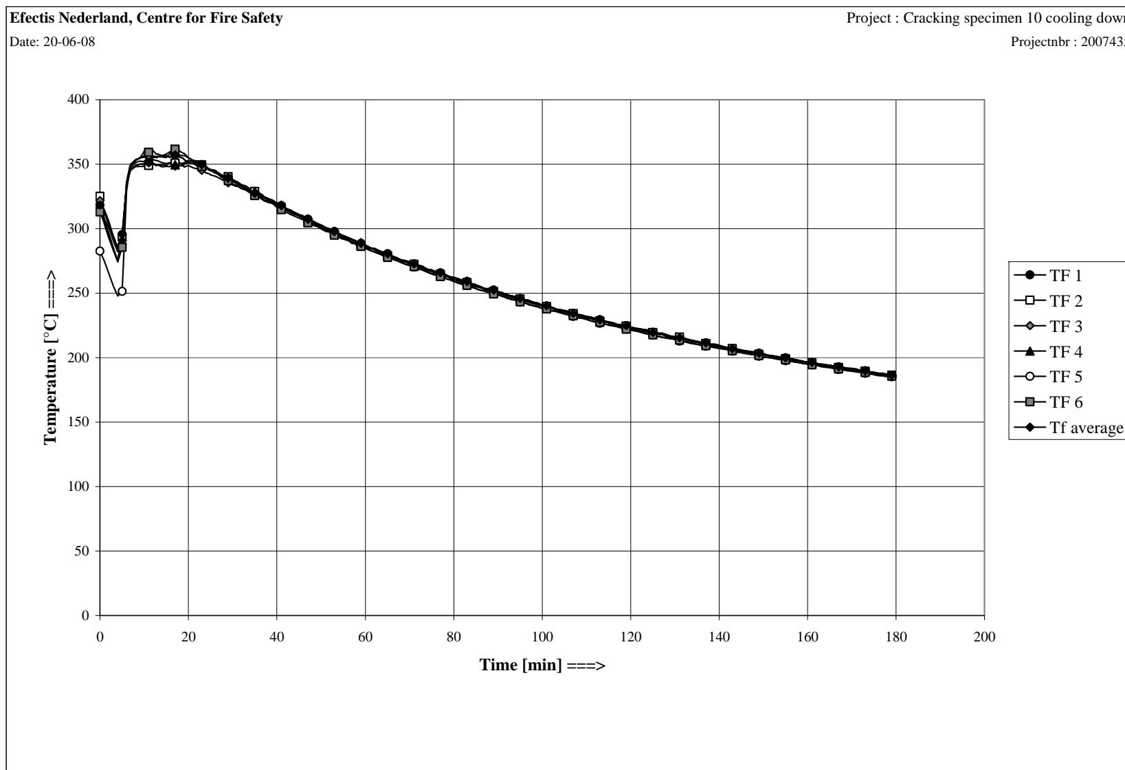
Figure C5 Furnace temperature during cooling down
