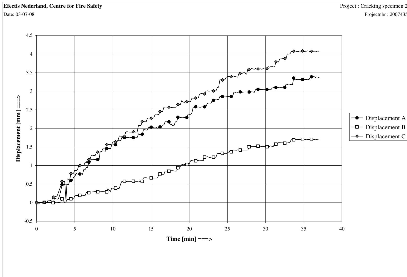
Figure F3 Displacement of the cold surface
