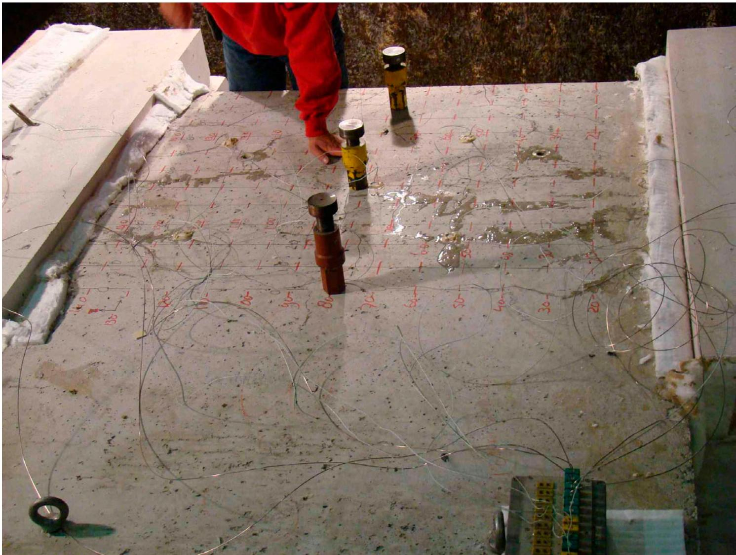
Figure D9 Element 8 after 15 minutes of heating
