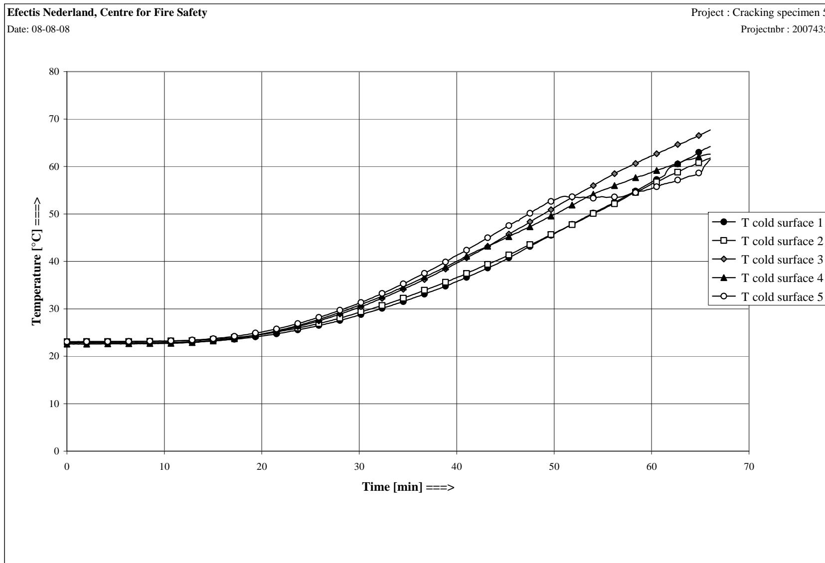
Figure H2 Cold face temperatures
