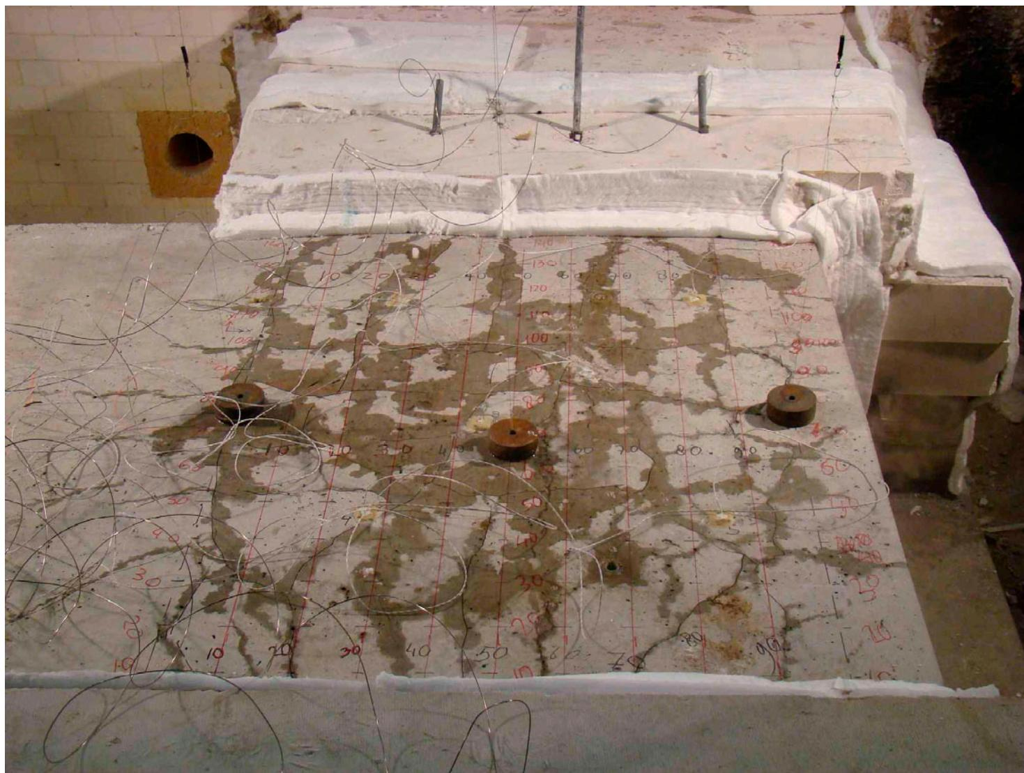
Figure G12 Element 9 directly after the fire test
