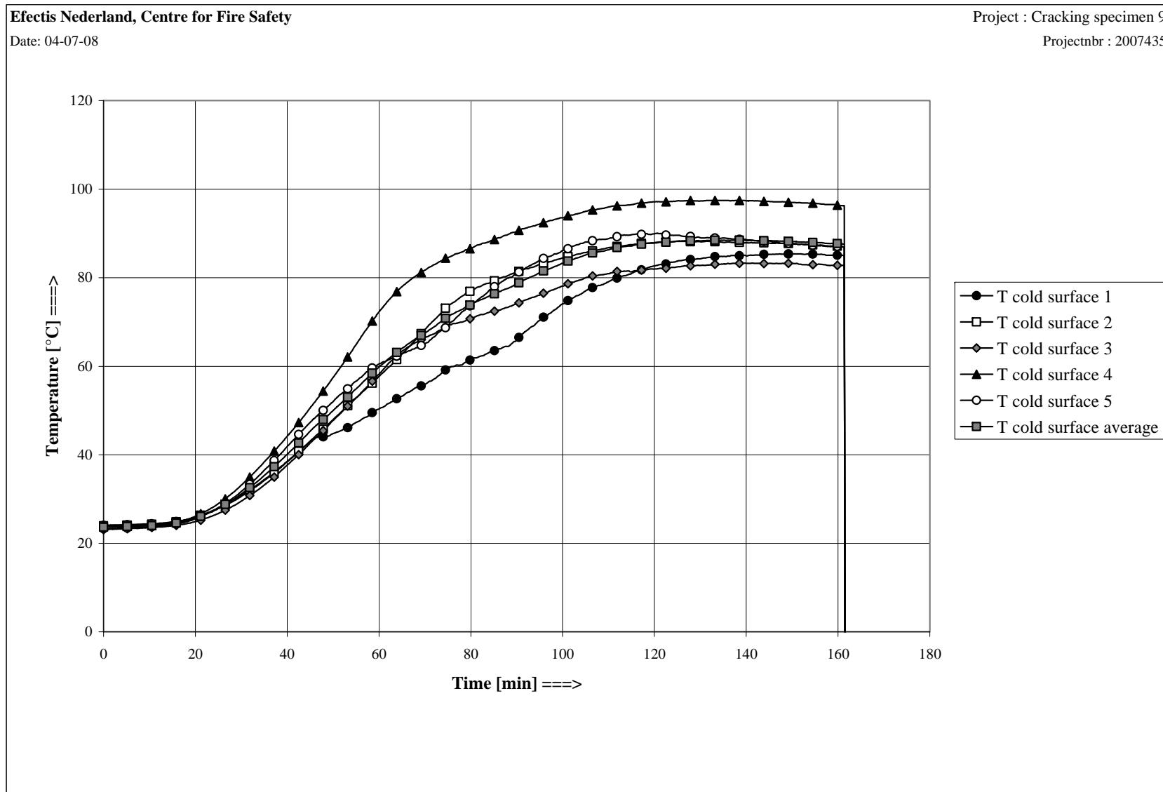
Figure G2 Cold face temperatures
