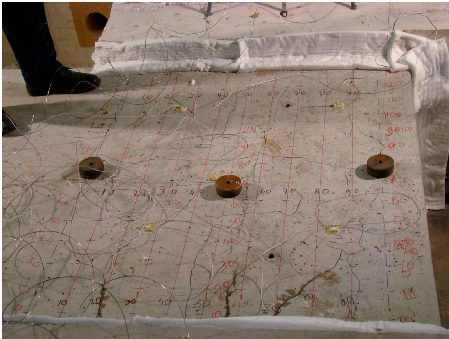
Figure G9 Element 9 after 24 minutes of heating
