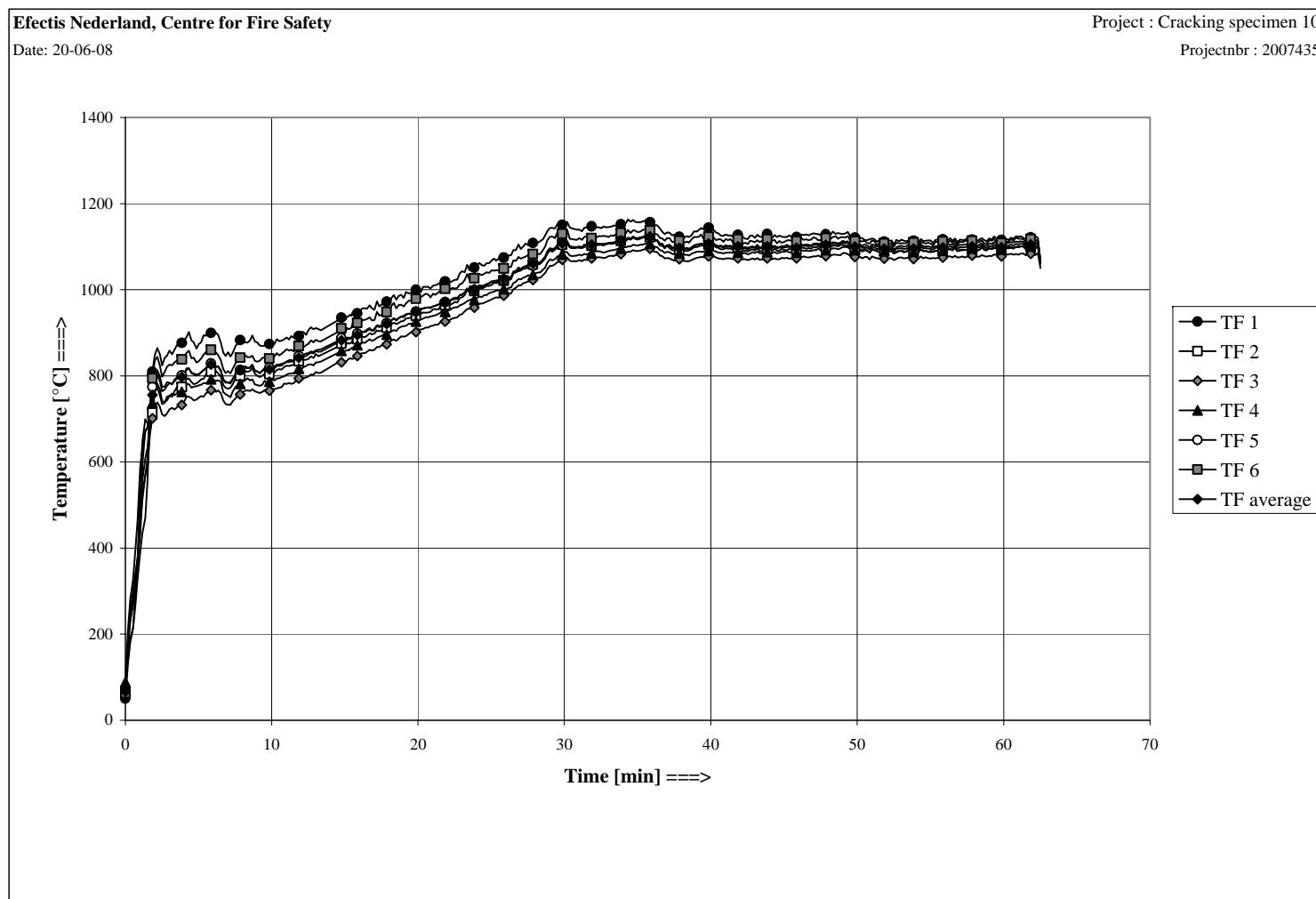
Figure C1 Furnace temperature
