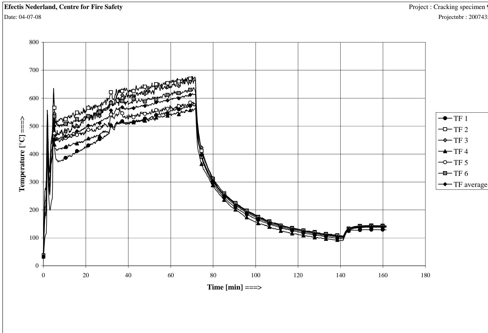
Figure G1 Furnace temperatures
