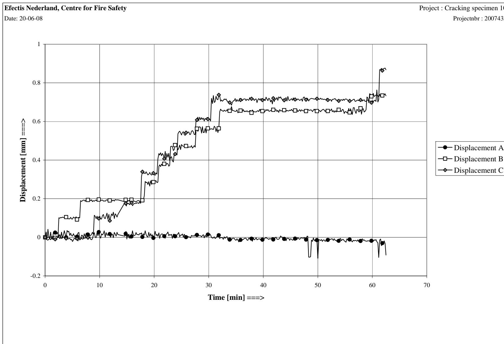
Figure C4 Displacement of the cold surface
