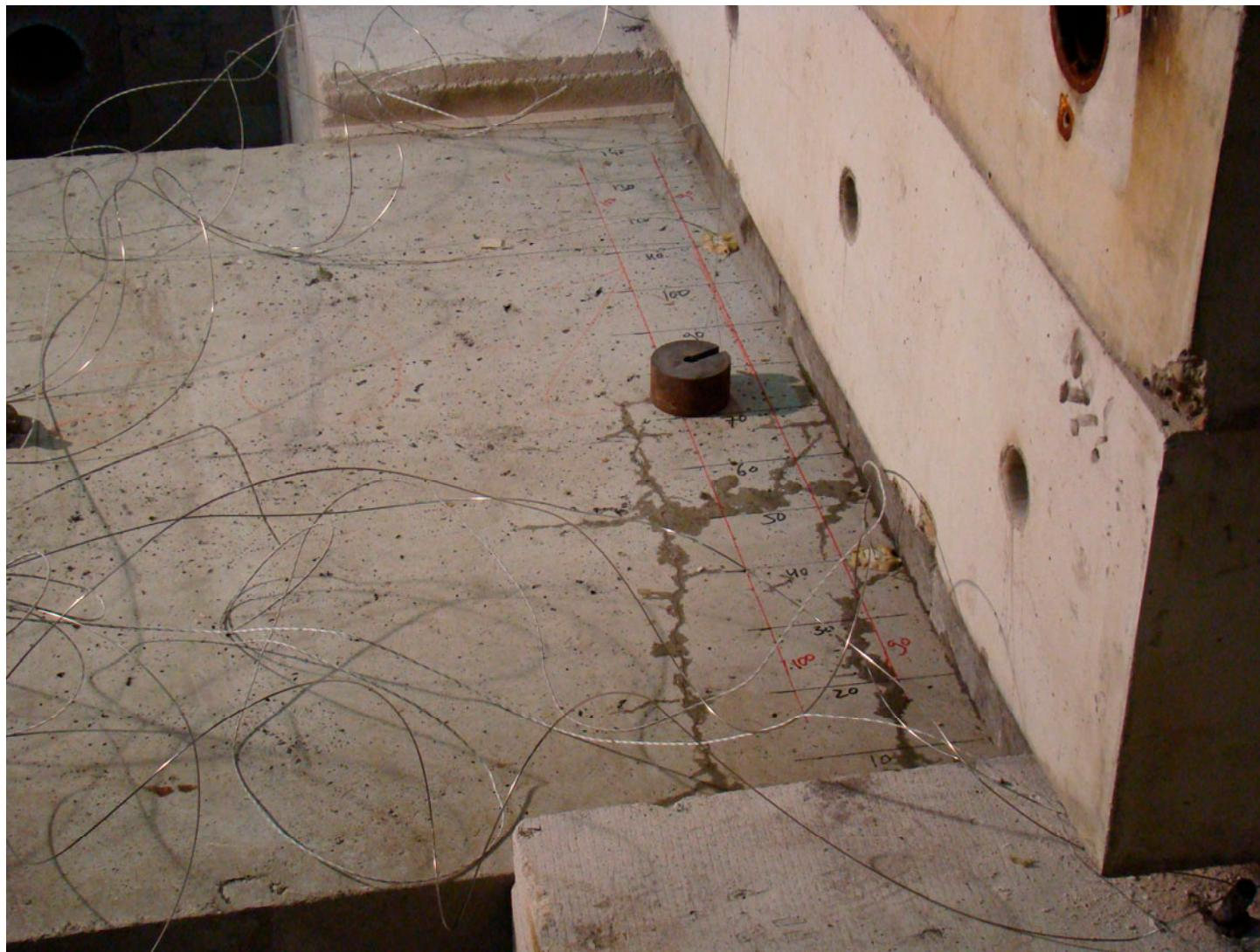
Figure I7 Element 7 after 50 minutes of heating, a view on the middle wall
