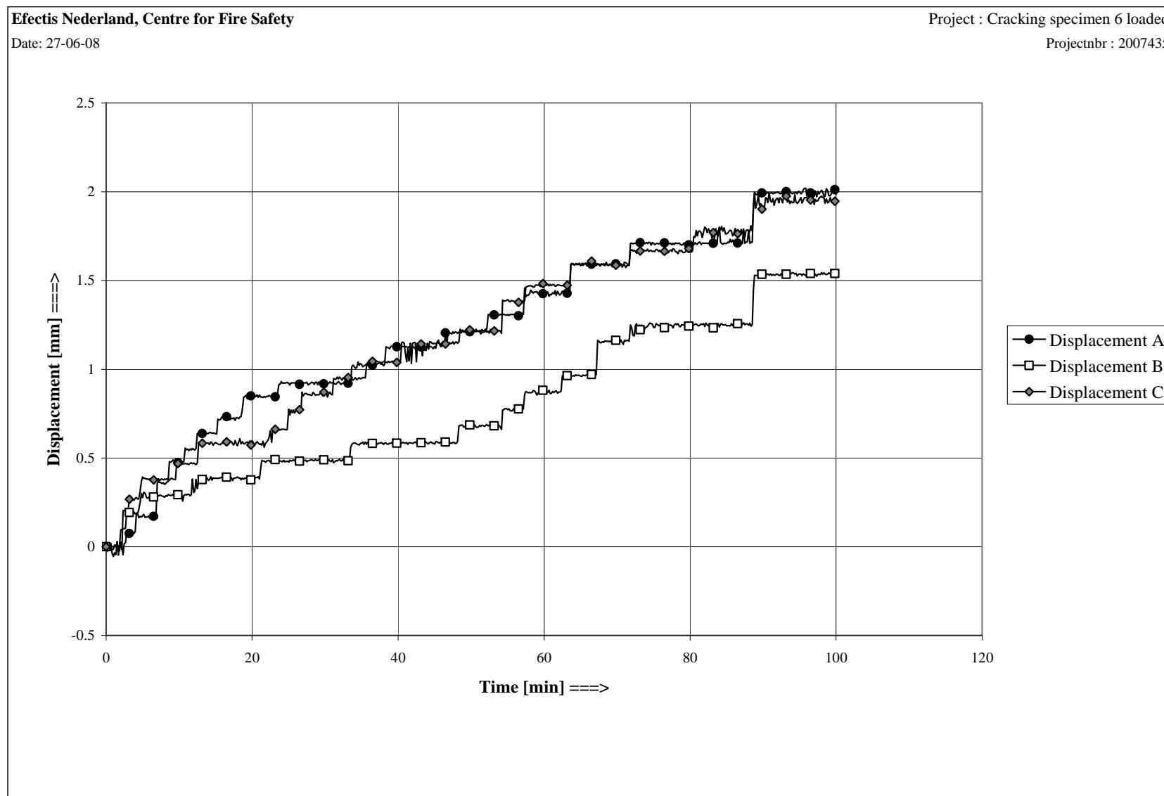
Figure E4 Displacements of the cold surface
