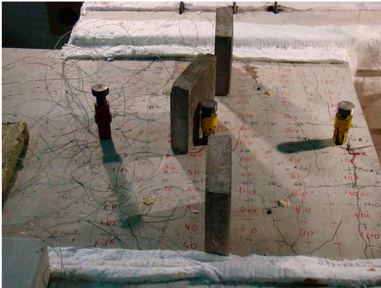
Figure C13 Element 10 after 48 minutes of heating
