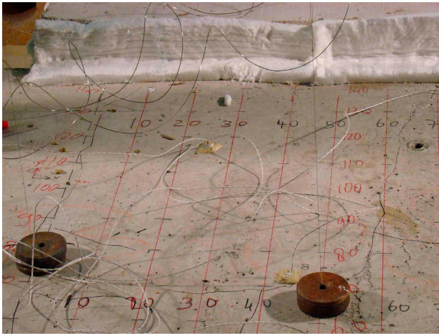
Figure G5 Element 9 after 14 minutes of heating, upper left corner
