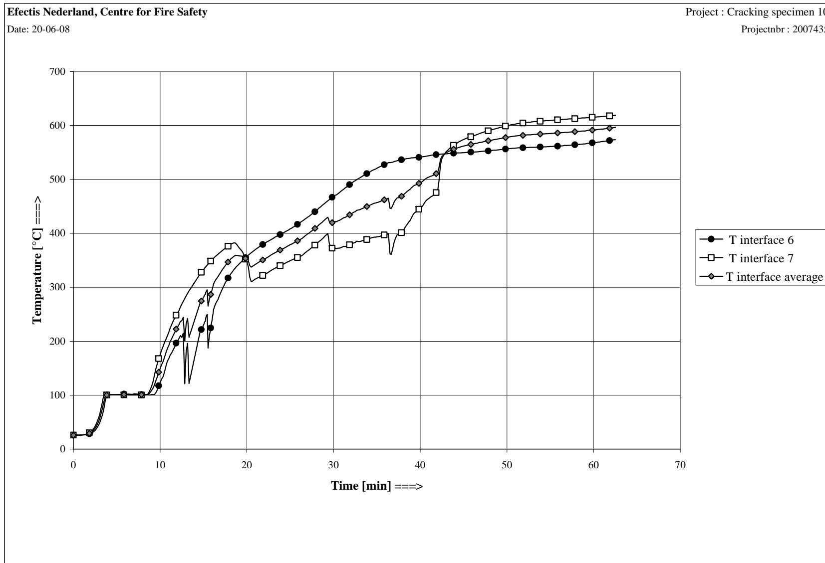
Figure C3 Interface temperatures
