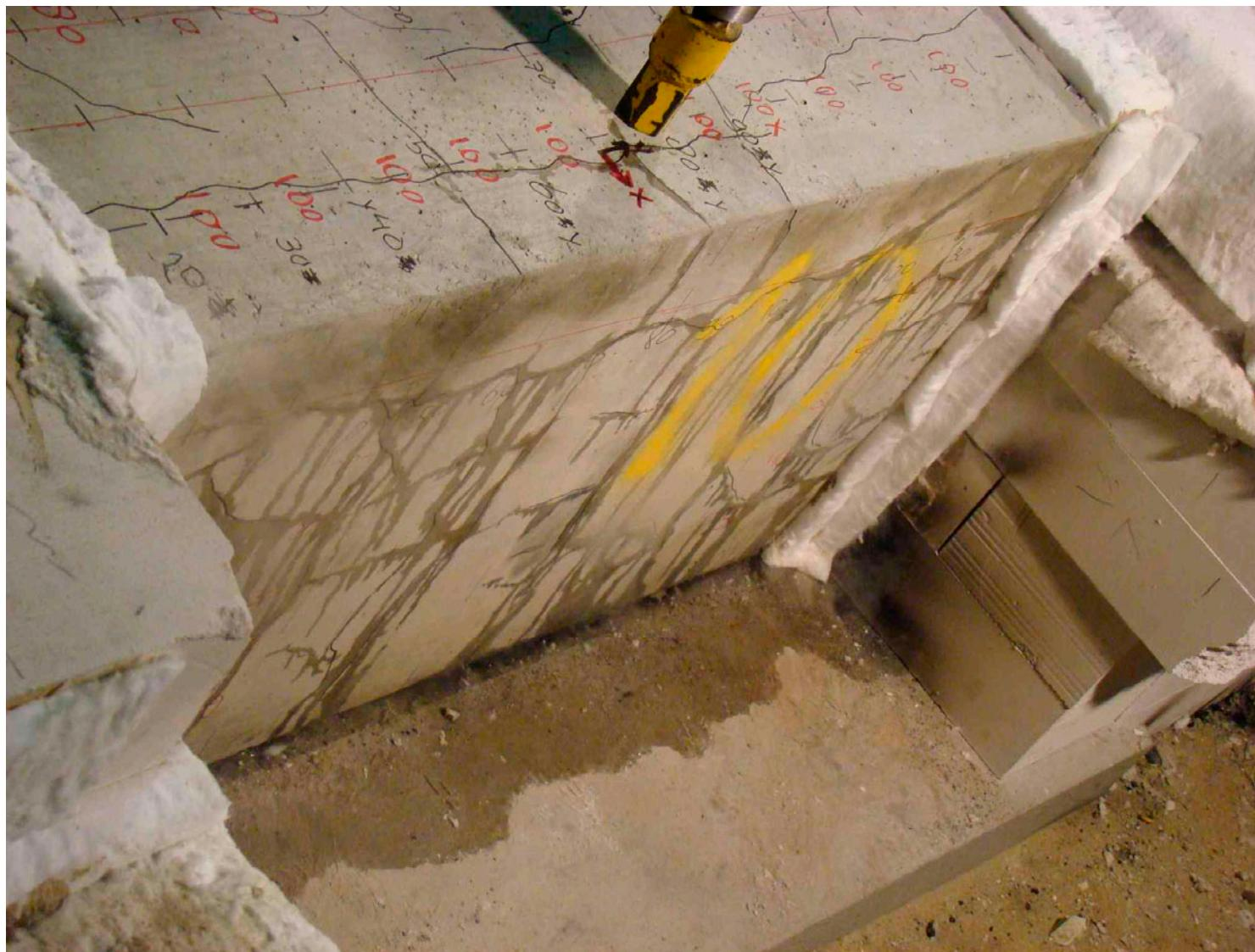
Figure C14 Element 10 after 48 minutes of heating, a view on the side surface
