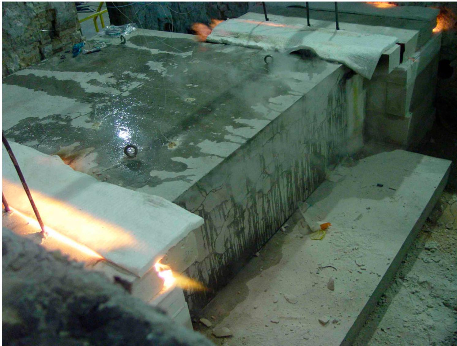
Figure A7 Element 0 after 29 minutes of heating
