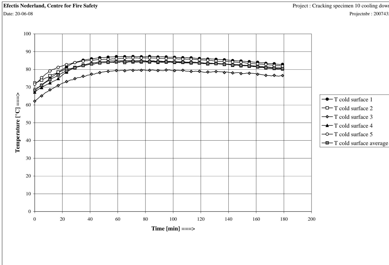
Figure C6 Cold surface temperatures during cooling down
